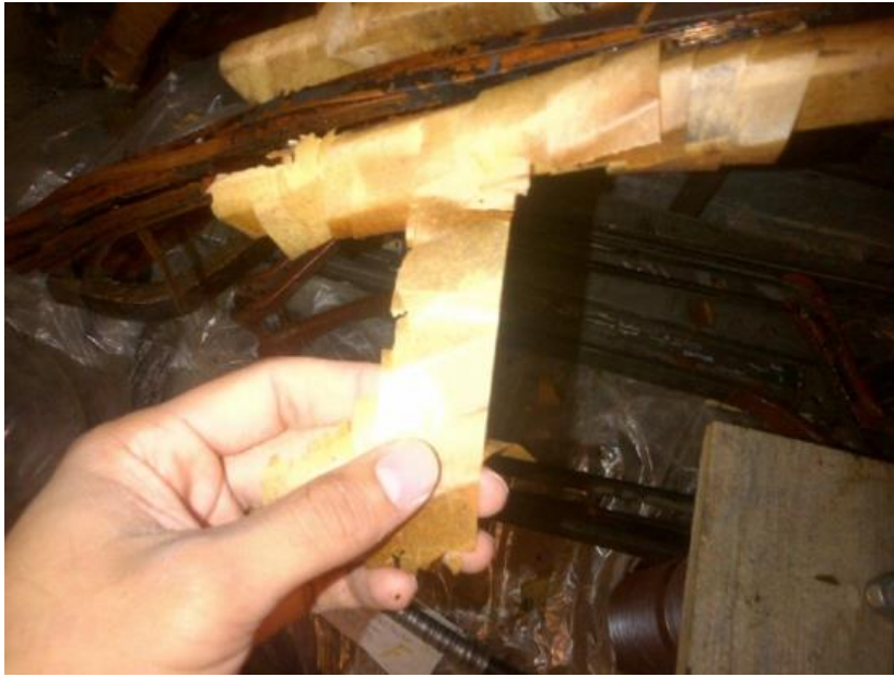
Figure 2.1. A power transformer insulation Kraft paper [4]
