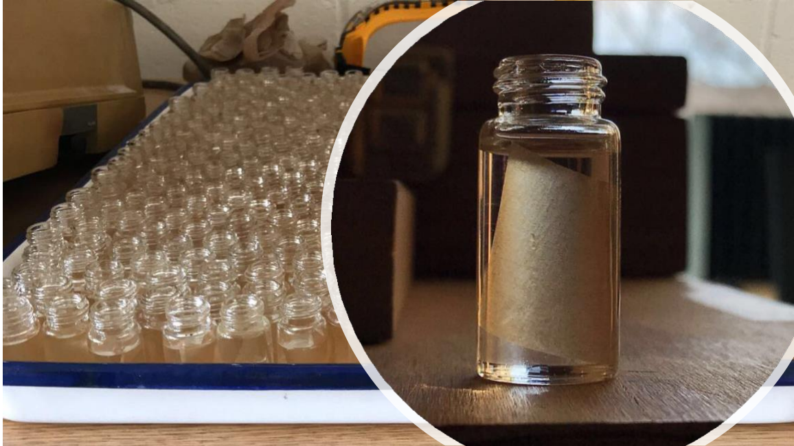
Figure 7.2. Sample vials containing Kraft paper and 10 ml of insulating oil.
