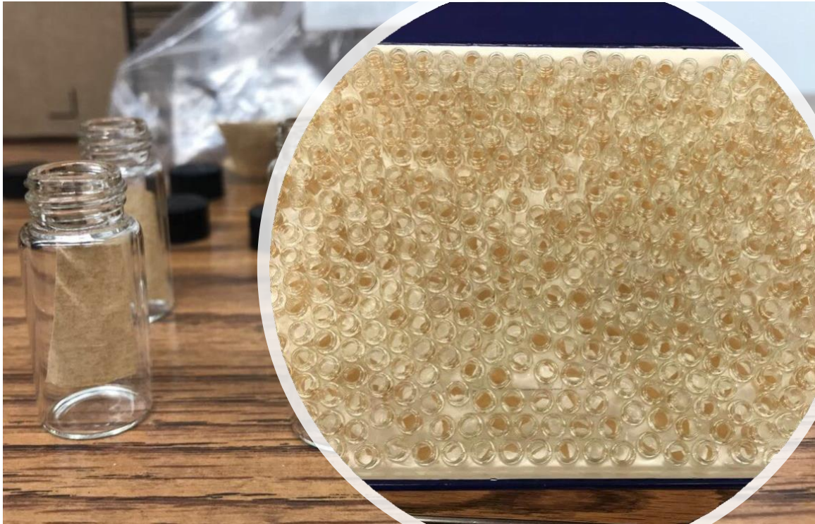
Figure 7.1. Preparation of sample vials containing Kraft papers for removal of pre-existing moisture.
