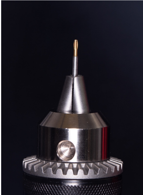
Figure 7. Nobel UniGrip driver (Nobel BioCare) attached to the Torque Meter (MTT03-05, Mark-10) through the Jacob's Chuck.
