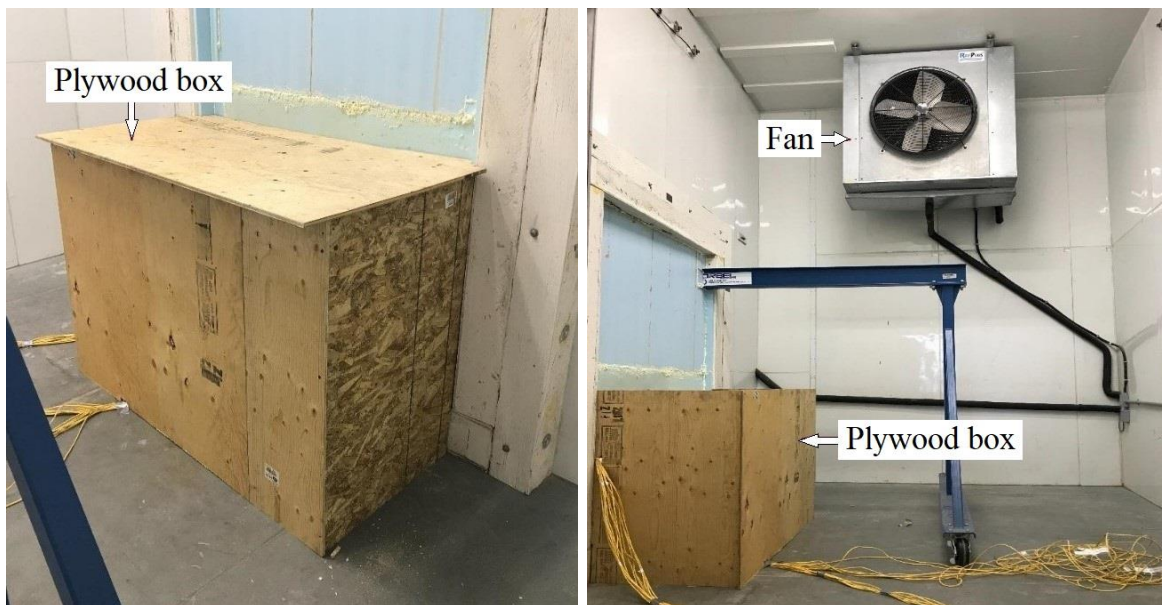
Figure 36 Plywood boxes to ensure uniform heat/cold distribution
