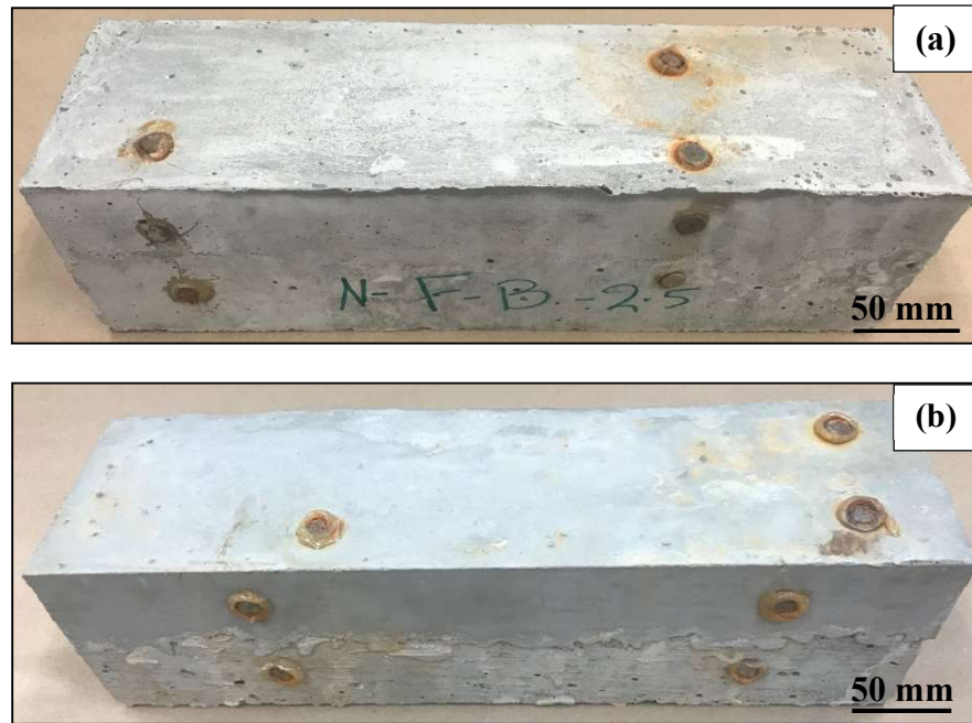
Figure 6.6: Exemplar surface conditions of the repair/overlay assembly after 180 days (56 days standard curing plus 124 days in hot/arid conditions); (a) N-F-2.5, and (b) N-G-2.5
