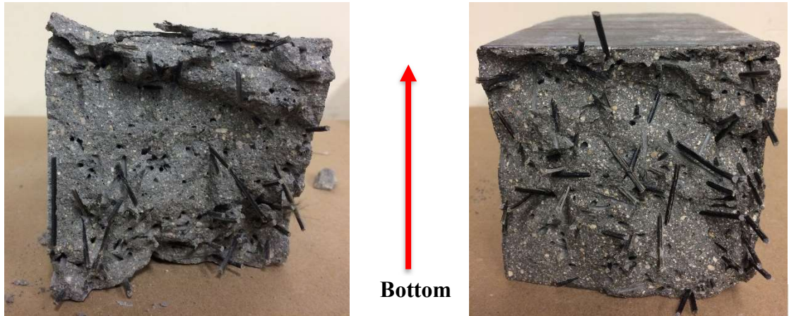
Figure 3.5: Distribution of BFP at the failure planes: (a) F-4.5, and (b) G-4.5.
