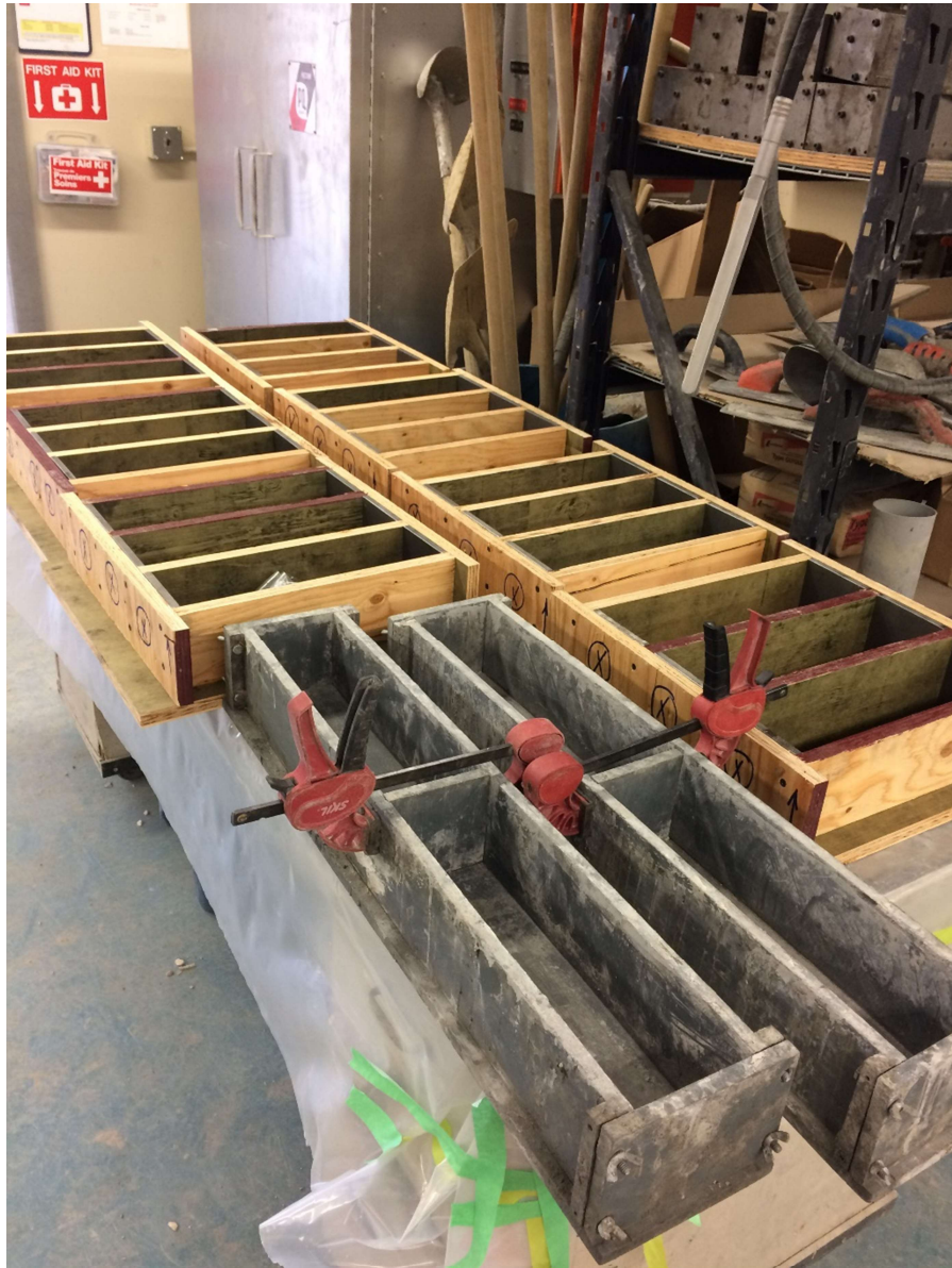
Figure C.1: Preparations and molds for the prismatic specimens of the different exposures.
