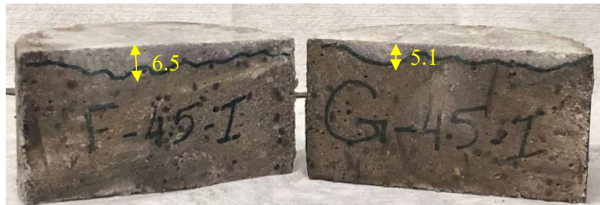
Figure 3.6: Whitish precipitate indicating the penetration depth of chloride ions into the F-4.5 and G-4.5 composites.
