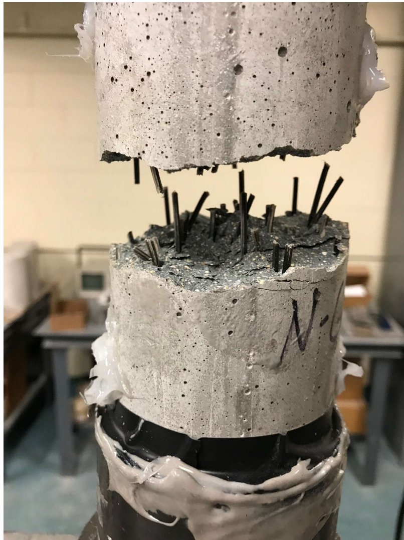
Figure B.3: Quasi-static tensile test specimen failure in the middle.
