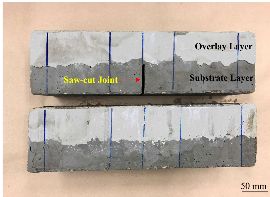
Figure 7.2: Exemplar overlay assembly for N-G-4.5 specimens.
