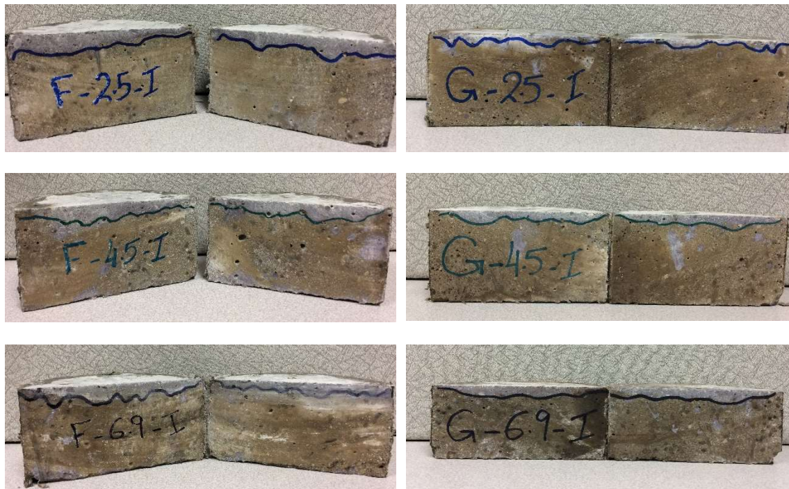
Figure A.5: Whitish precipitates show the average penetration depth of chloride ions for the developed composites
