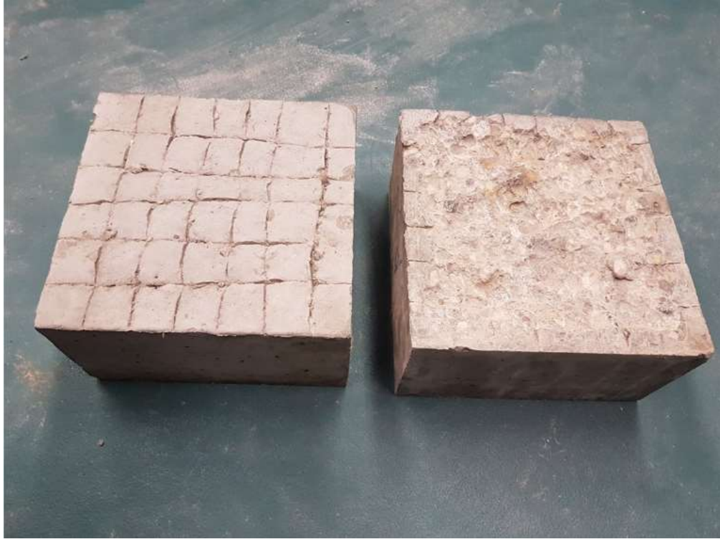
Figure D.2: Parent concrete surface before and after roughening
