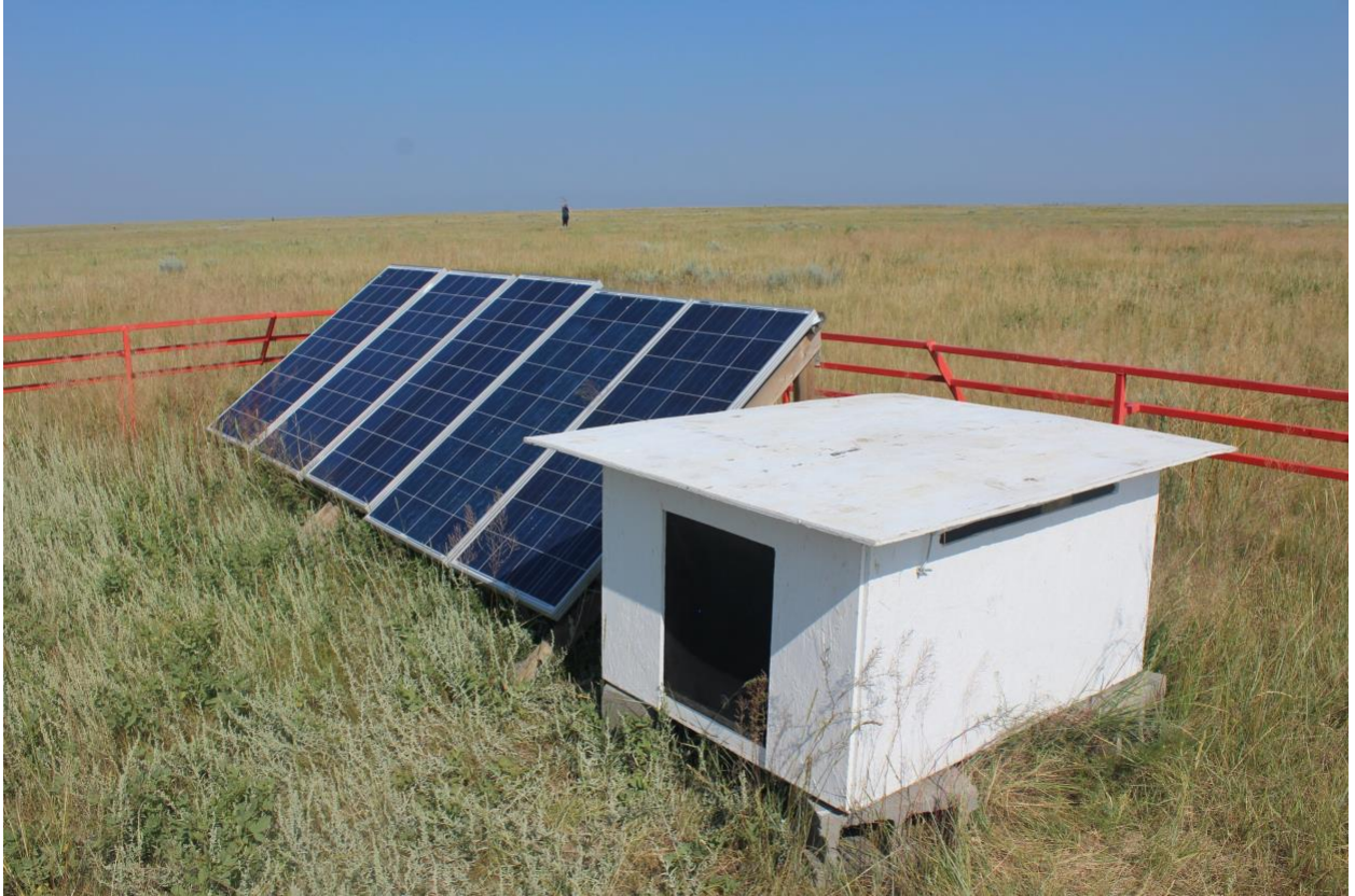
Figure 3 This image shows one active, noise broadcasting unit used for the experimental design. The infrastructure includes a wooden box housing batteries and electrical equipment, five solar panels, and metal fencing. Image from Hannah Carey 2018.
