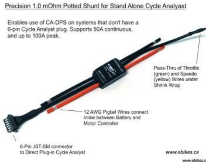
Figure 12 CA molded precision shunt
