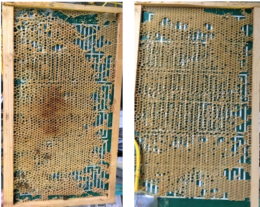
Figure 5.12- Capacitance board 2 frontside (right), backside (left). Picture taken October 3, 2018.
