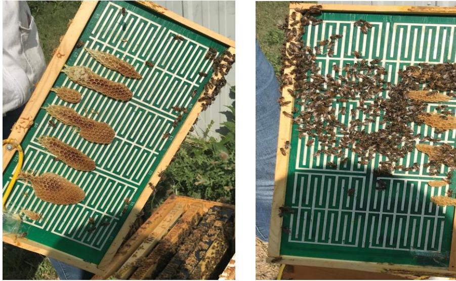
Figure 5.5- Capacitance board 2 frontside (right), backside (left). Picture taken August 22, 2018.
