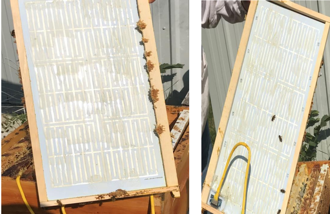
Figure 5.9- Capacitance board 6 frontside (right), backside (left). Picture taken August 22, 2018.
