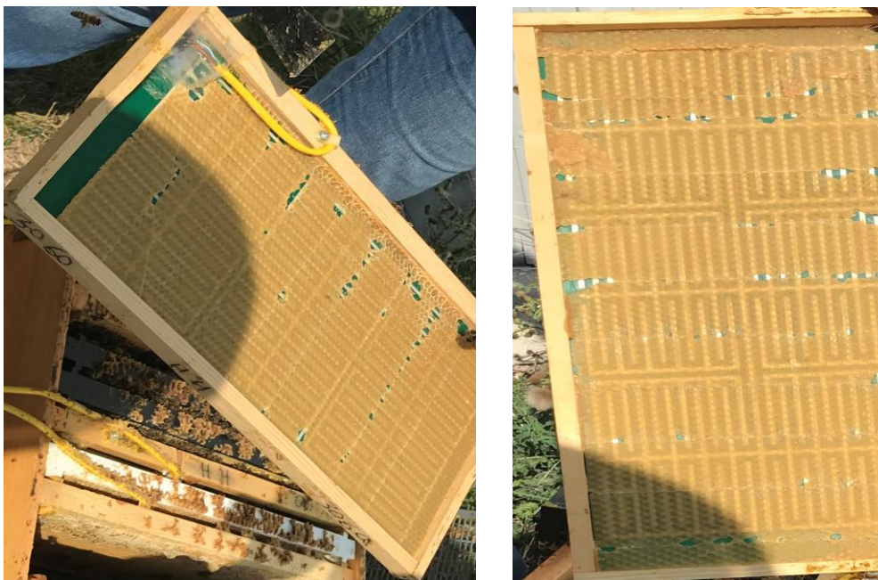
Figure 5.6- Capacitance board 3 frontside (right), backside (left). Picture taken August 22, 2018.
