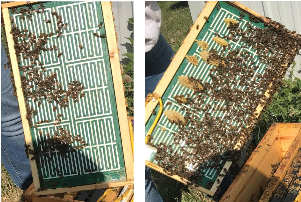
Figure 5.4- Capacitance board 1 frontside (right), backside (left). Picture taken August 22, 2018.
