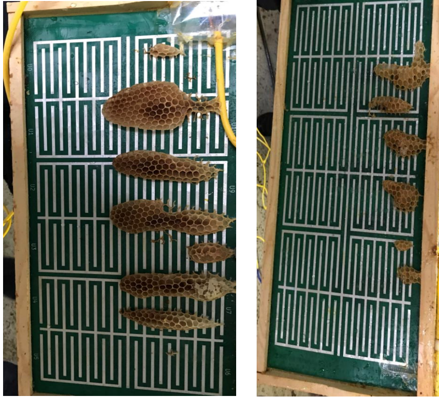
Figure 5.12- Capacitance board 2 frontside (right), backside (left). Picture taken October 3, 2018.
