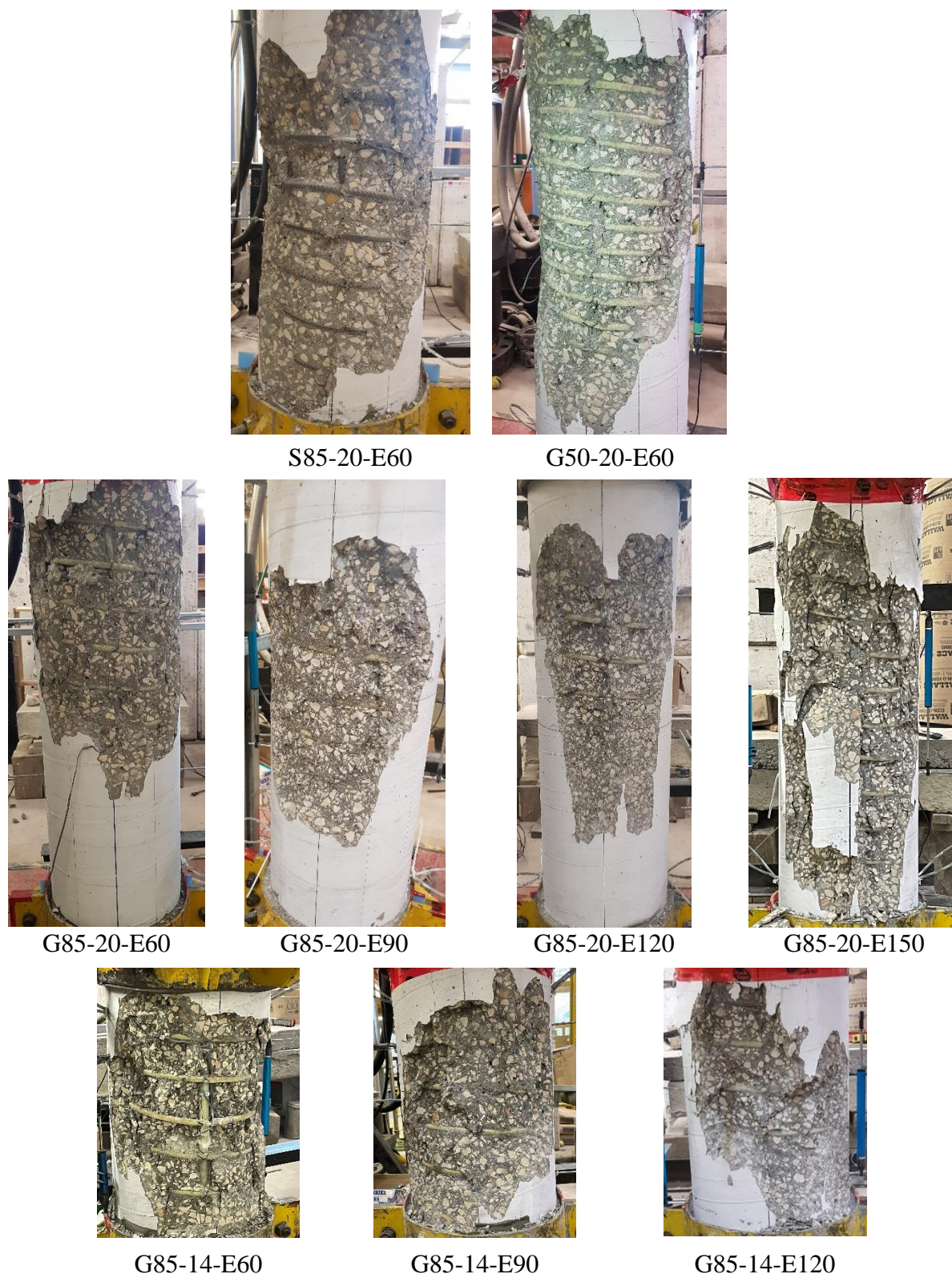
Figure 5.3 – Mode of failure for axially-loaded columns
