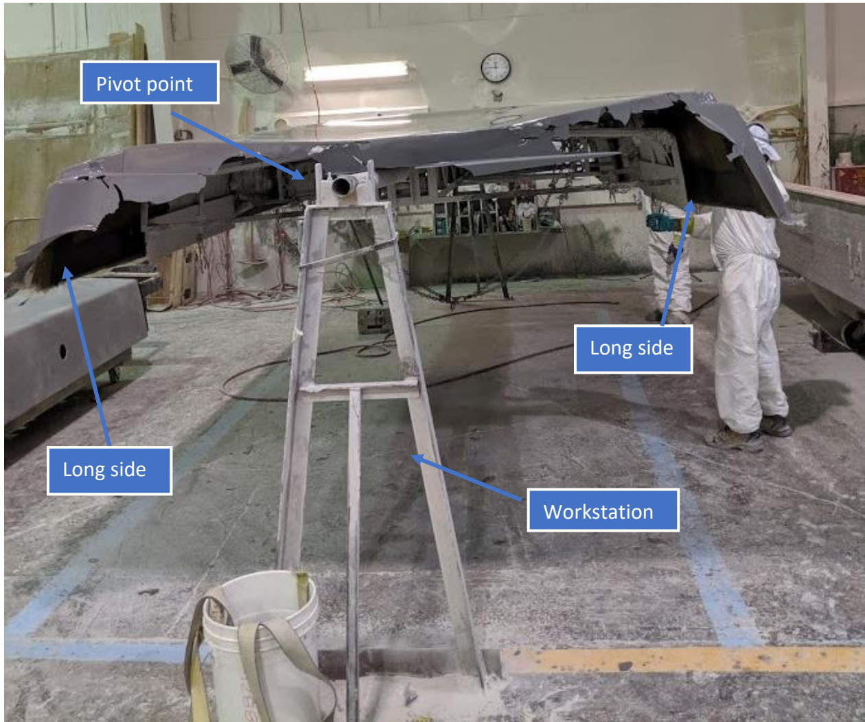
Figure A-3: Workstation 1, trimming and sanding of the sides (taken with permission)
