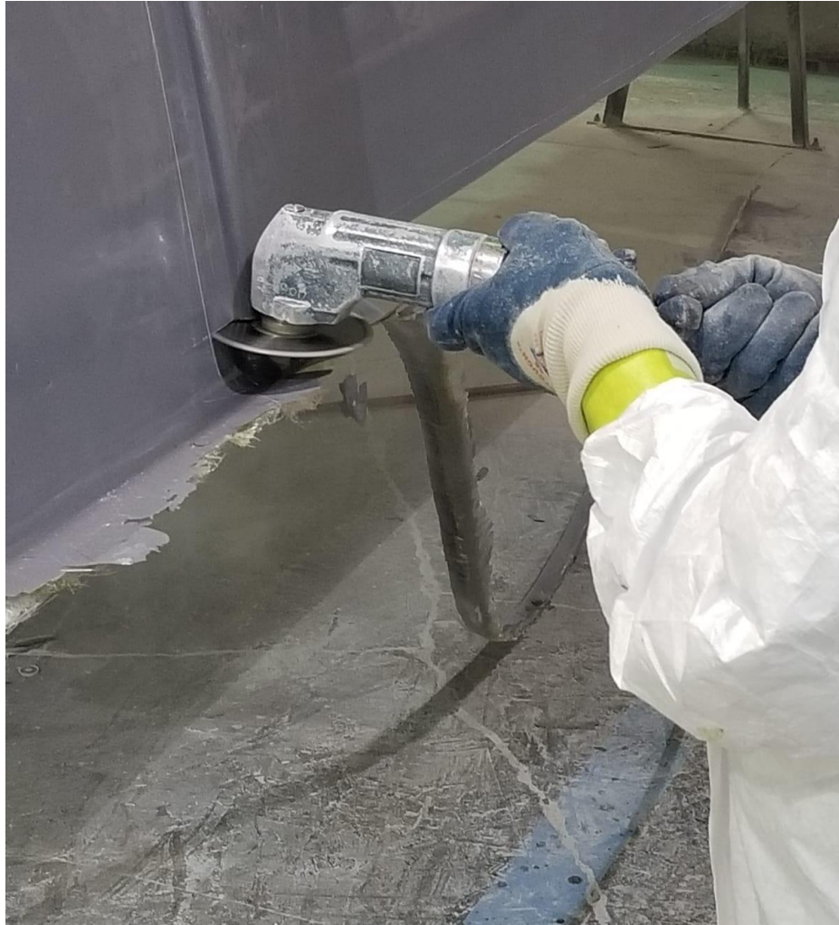
Figure 1: Operator cutting a roof component, while being exposed to the cutting blade (taken with permission)
