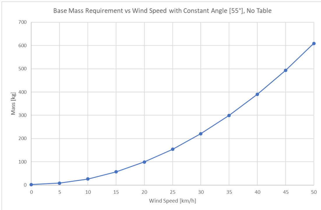
Figure 13: Base Mass Requirement for Constant Angle, Variable Wind
