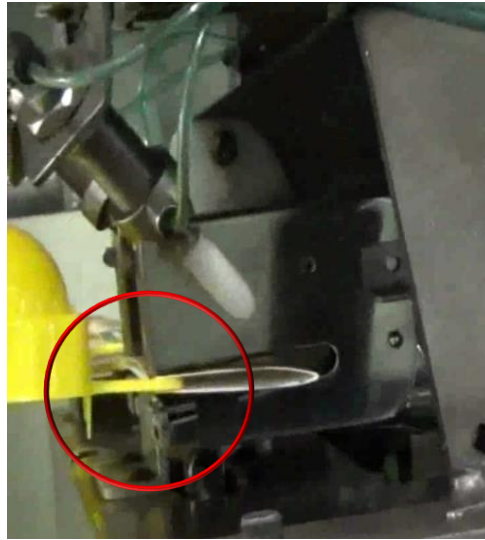
Figure 3: A header card located incorrectly on the egg holder handle resulting in the stapler stapling into the handle [5].
