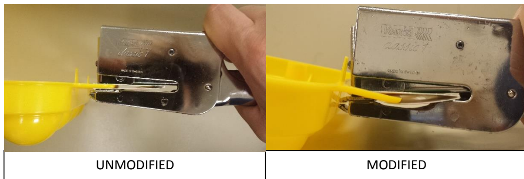
Figure 7: Comparison of unmodified and modified stapler stapling the egg holder. Note the modified stapler is able to completely close while the unmodified stapler is capable of closing only part way [12].
