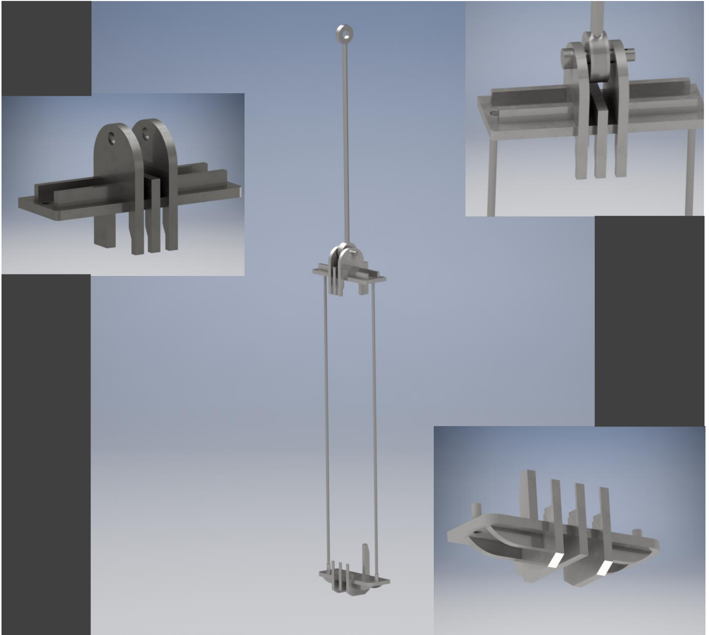
Figure 6: Full assembly of existing lifting device. Inset, clockwise from left: The top clamp; the top clamp assembly with the lifting hook attached by pin; and the bottom clamp
