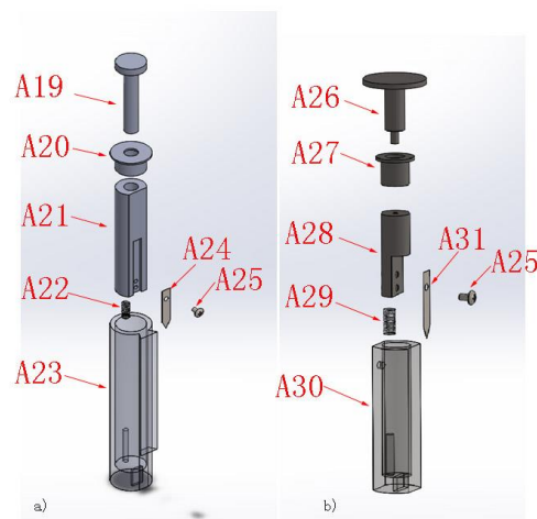
Figure 18 – Exploded View of Cutting Pens A and B
