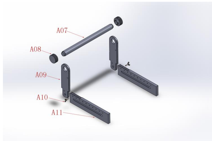
Figure 16 – Exploded View of Mylar Roll Holder
