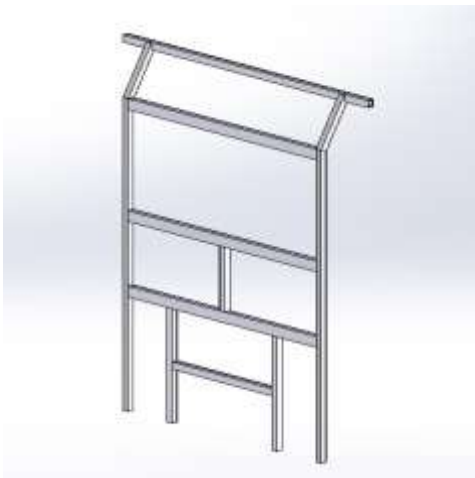
Figure 4: Refined subassembly. All extraneous modelling features have been suppressed. Component interferences have been resolved.
