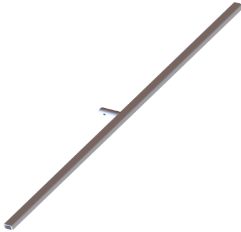
Figure A-19: Square tubing for upper frame
