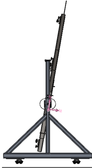
Figure 23: Side view of the Centre of Gravity for Device
