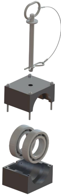
Figure A-16: Rotational mechanism with pin
