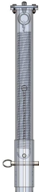
Figure 20: Internal renders of the spring mechanism
