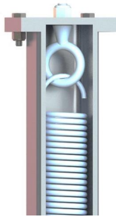
Figure 18: Mounting of the extension spring to the eye bolt
