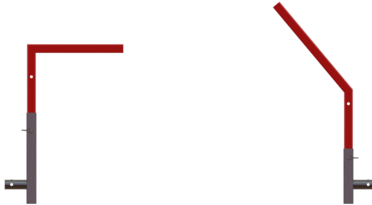
Figure 14: Adjustable top members of the upper frame assembly
