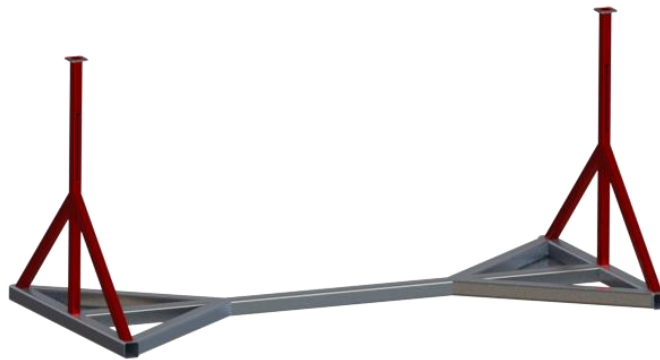
Figure 5: Bottom frame showing highlight to vertical members
