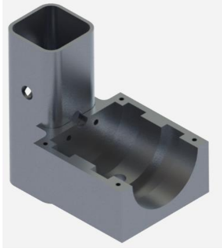
Figure 9: Isometric view of slider sleeve and lower rotational block
