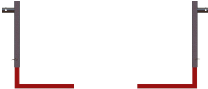
Figure 13: Fixed bottom members of the upper frame assembly
