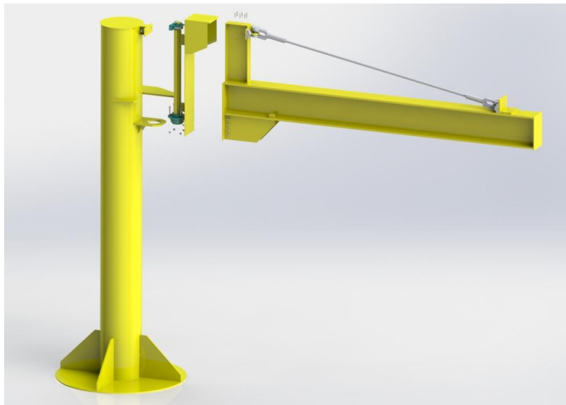
Figure D15 Exploded jib crane.
