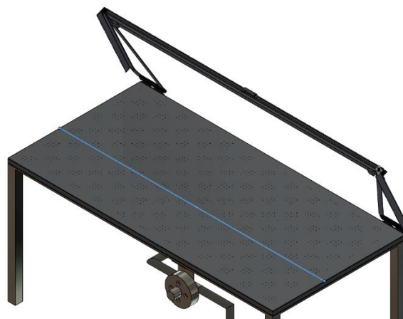
Figure 19: Calibration line on vacuum table for eye mark alignment.
