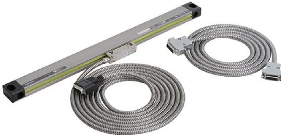
Figure 7: Mitutoyo® ABS AT715-1700 linear scale [4].
