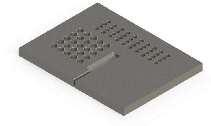
Figure 24. Isometric view of the downdraft table CAD model
