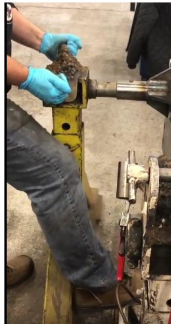
Figure A12: Disconnecting the A-Stand from the Welding Fixture
