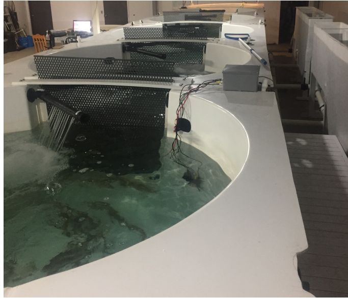
Figure 4.3: Side-view of the fish tank (left of walkway). Sensor pack B is seen in this photo, with its probes submerged in the tank. To the right of the walkway, the settling tanks.
