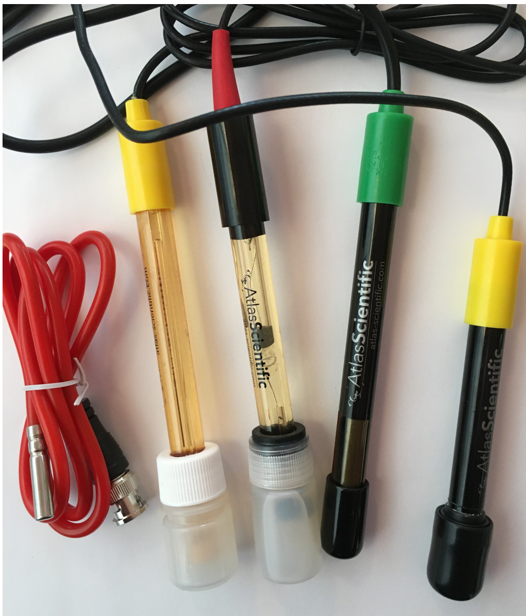
Figure A.4: Atlas Scientific EZO probes. From left to right, temperature, ORP, pH, EC, and DO.
