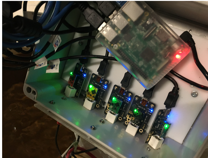
Figure 4.6: Inside the sensor pack, the Raspberry Pi is shown, as well as the 5 EZO sensor boards interfaced via a USB carrier board.
