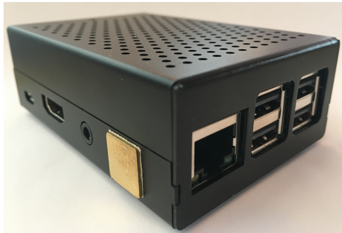
Figure A.3: The Raspberry Pi 3 is the brain of the sensor pack. It is an ARM-based micro computer which runs a custom distribution of Debian Linux, called Raspbian. It is responsible for gathering readings from the sensors and relaying them to the central server.
