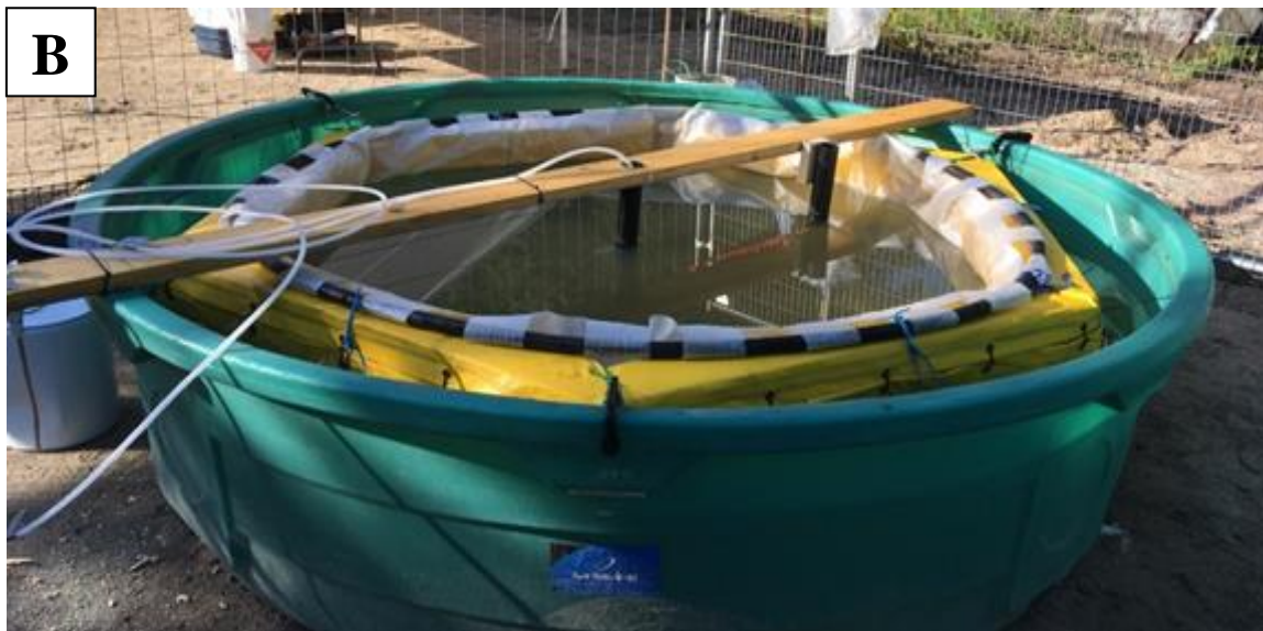
Figure 3.1: (A) Vertical profile of microcosm used in pilot-scale study in August 2017 at IISD-Experimental Lakes Area. (B) Microcosm consisting of an outer containment tank, Novathene microcosm wall secured to a yellow flotation collar via flexible tubing, with sampling ports stretching across tank.
