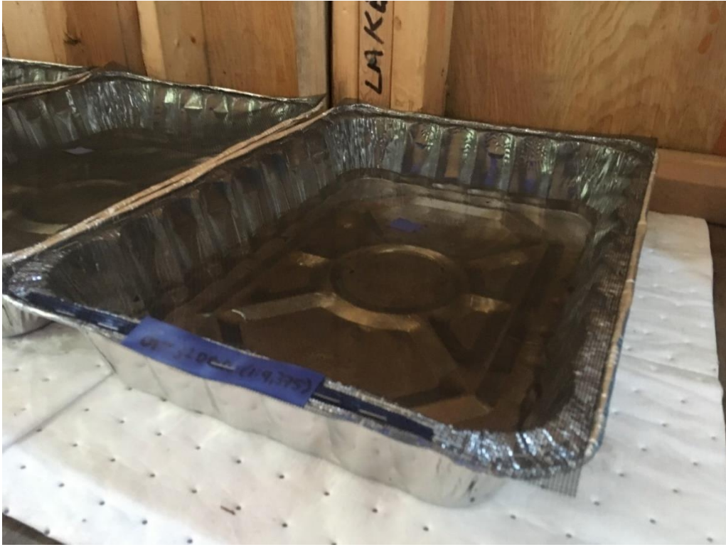
Figure 3.12: Test vessel used in evaluating impacts of surface sheen exposure of Cold Lake Winter Blend diluted bitumen to surface-dwelling freshwater bugs (water striders; Family: Gerridae).
