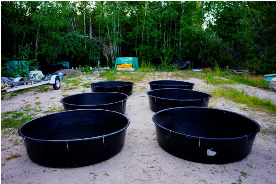
Figure 3.14: Large tanks used to conduct the large-scale exposure to fresh Cold Lake Winter Blend diluted bitumen evaluating impacts of surface sheen exposure to surface-dwelling freshwater bugs (water striders; Family: Gerridae). Tanks were 1.7 metres in diameter and contained 220 litres of water each. Oil added ranged from 0 uL to 460 uL (0 drops to 81 drops of oil).
