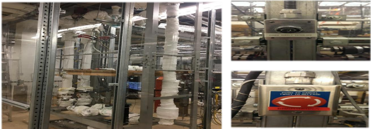
Figure 3.9: Safety features of SFF-V (in picture: Perspex glass enclosure, safety key and emergency stop button)
