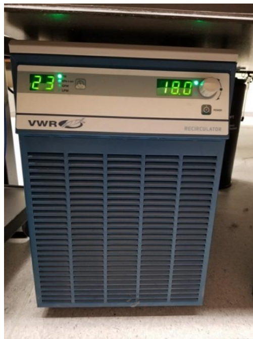
Figure 3.3 Recirculating water chiller of the cooling system for laser. Digital displays show both the room temperature (to the left) and the temperature of the water in the cooling system (to the right) as at time of snapshot
