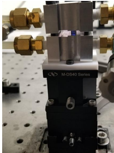
Figure 3.2 Crystal cooling arrangement. Indium foil-wrapped-crystal (tiny blue material) sandwiched in metal holder
