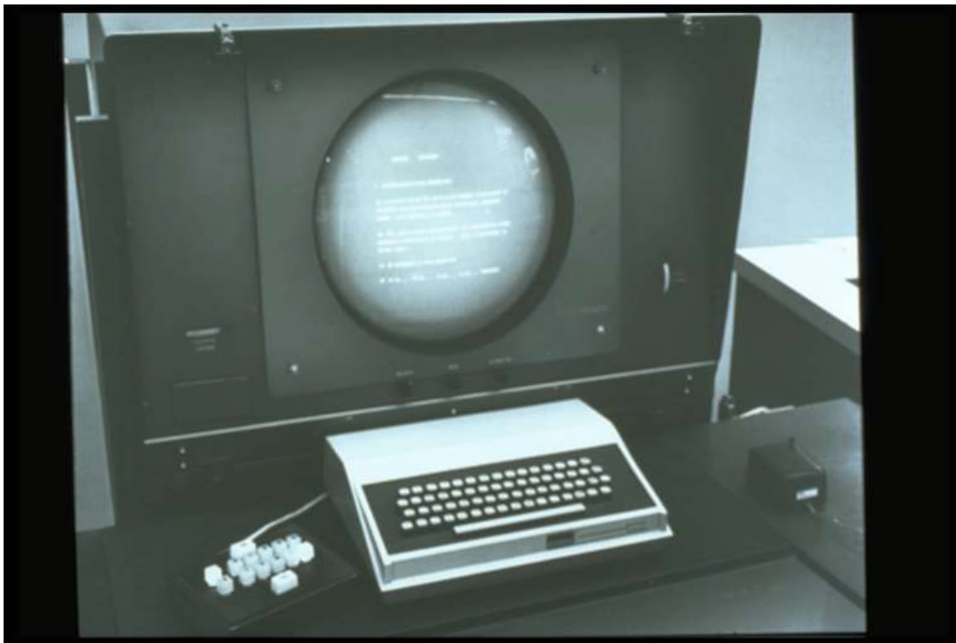
Figure 2: "The on-line system workstation showing the CRT display, keyboard, pushbuttons, and mouse." 55
