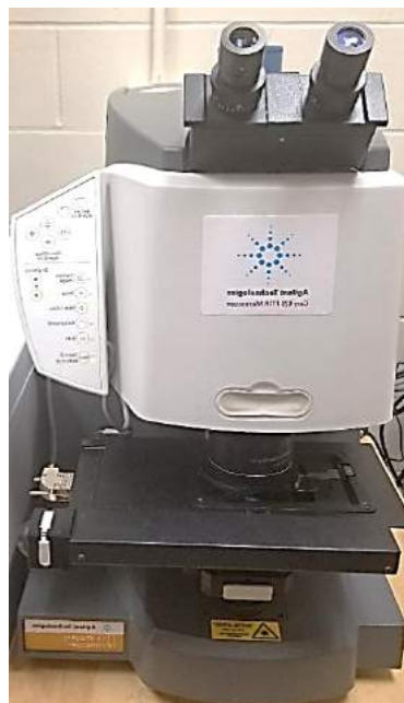
Figure 3.4. A- The Agilent-Cary 620 FTIR Microscope and 670 spectrometer used in this thesis.
