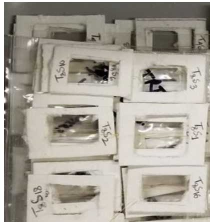
Figure 3.4: Fibres attached to the frames by glue
