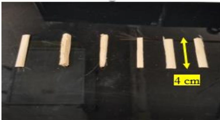
Figure 3.2: Leaves cut in 5 cm length for fiber extraction.
