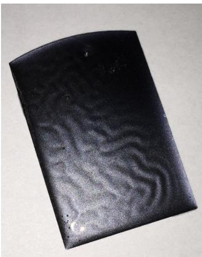
Fig. 6. 2. Large wrinkles appear on the spun SU-8 surface due to solvent trapped in the inner layers of the coated SU-8.
