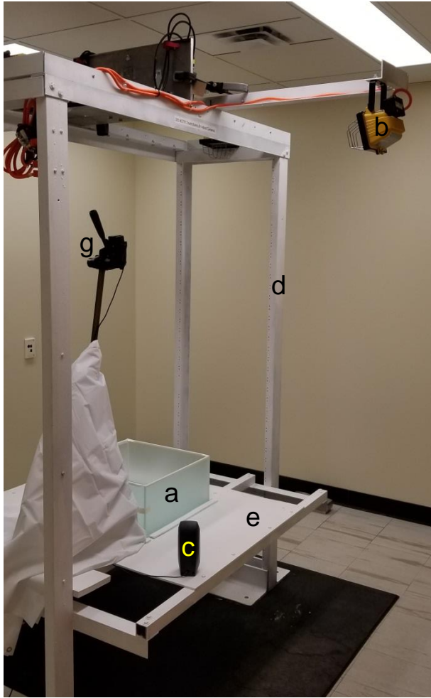
Figure 2. Images of experimental apparatus. Several aspects of the apparatus can be observed including (a) experimental tank (ET), (b) work lights, (c) speakers, (d) metal scaffolding, (e) white platform, (f) cameras, and (g) video camera. Photos by Brittany Cook, June 3, 2019.
