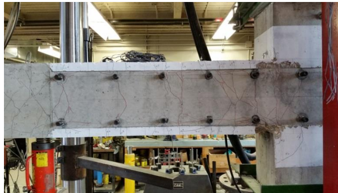
Figure 8.13 - Crack propagation in Specimen G-M after the first loading phase
