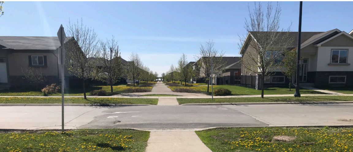
FIG 4.82 Left. This is a view down a large loop in Bridgwater Forest. The street is so long that you cannot see where it turns around. Long, straight streets encourage fast driving on residential roads.
