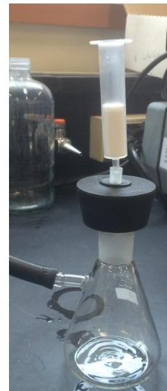
Figure 3: Set up for methanol rinse of the SPE cartridge
