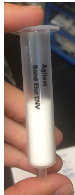
Figure 1: SPE cartridge used for fractionation
