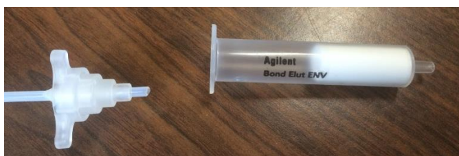
Figure 5: Image of an SPE cartridge, cap, and tube prior to assembly
