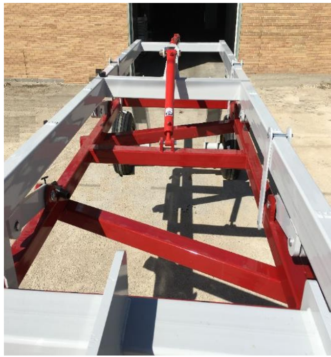
Figure 5.3 Manufactured field-testing unit with groove plate (a), hydraulic stoppers (b) and support plates (c).
