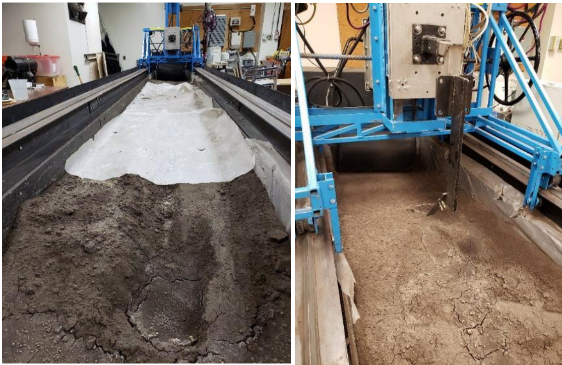
Figure 2.3 a) soil bin setup b) subsoiler tool attached to the soil bin carriage
