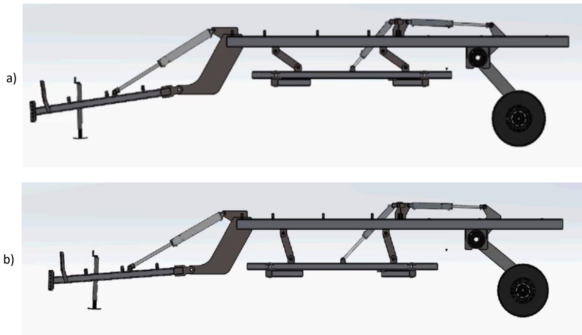
Figure 5.4 a) Field-testing unit with extended front and back hydraulic cylinder, b) Field-testing unit with extended subframe for opener field test.
