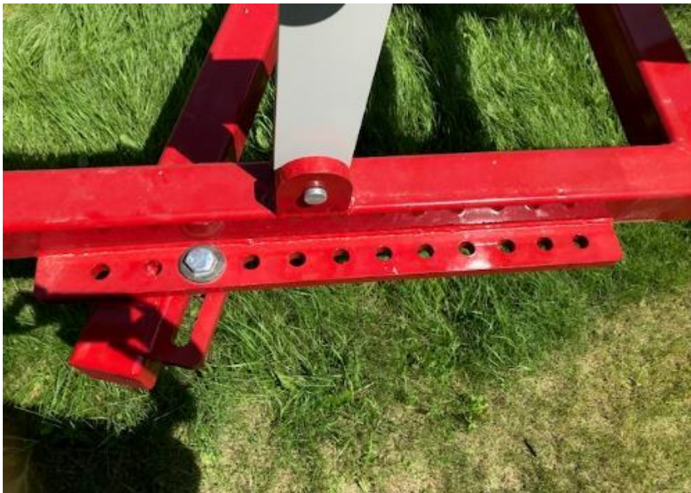
Figure 5.2 Gang angle adjustment mechanism connecting subframe and toolbar
