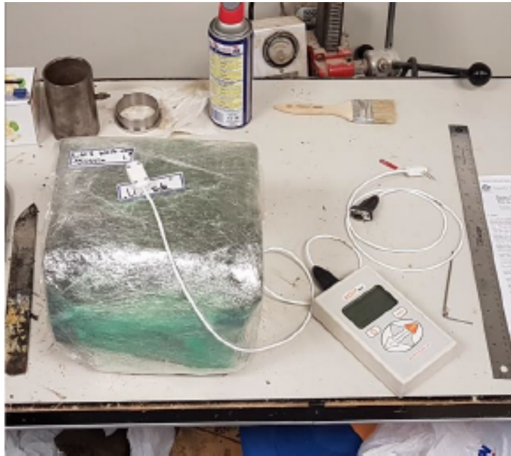
Fig. 2.4: Disturbed sample during thermal conductivity measurement test [16].
