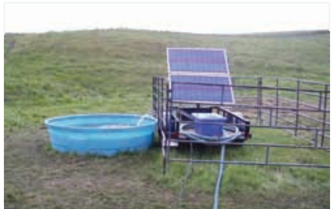
Solar-powered pumping systems allow producers to water cattle away from the stream.
