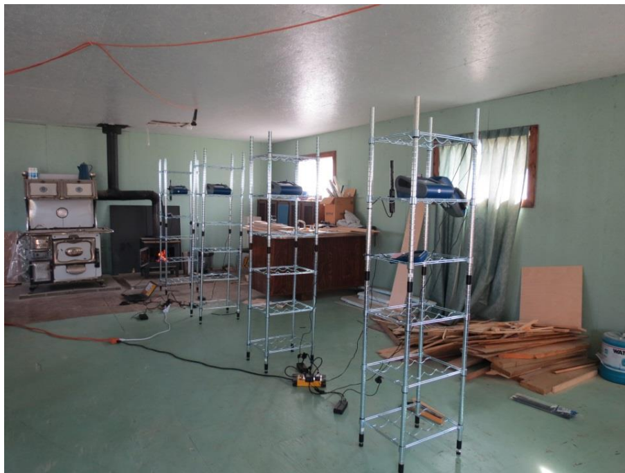
Figure 3.2. Location of Instruments Used to Monitor PM 2.5 Distribution at 4'-5.5" Above Floor Level and at Various Distances from the Woodstove
