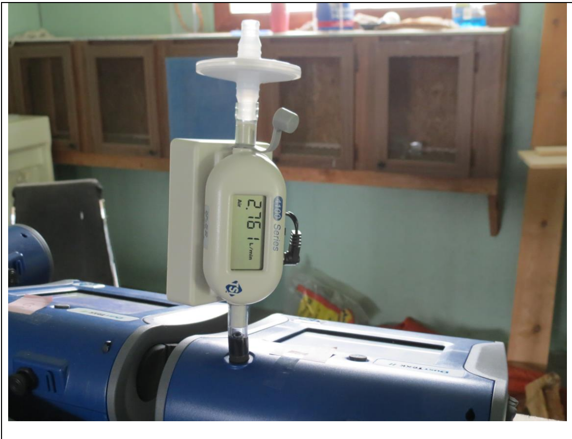
Figure A.2. Using a Flowmeter, Model TSI 4140, to Check the Flow Rate of the Dusttrak II Instruments
