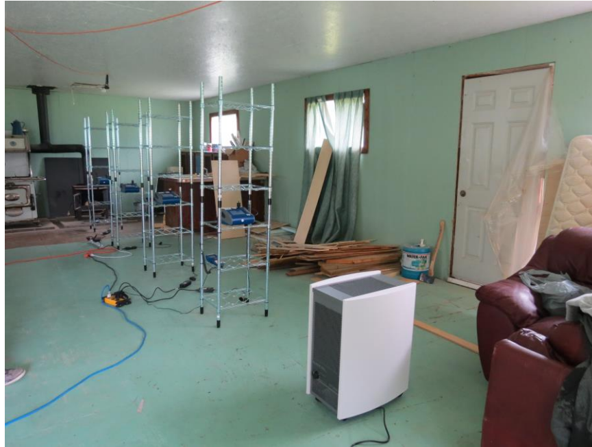
Figure 3.4. Set-Up Used to Determine PM_{2.5} Distribution at Various Durations of Time that the Woodstove Door Was Kept Open and with the Use of an Air Purifier
