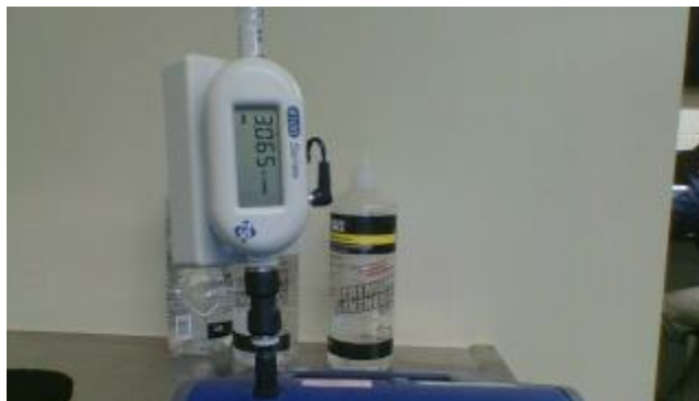
Figure B.4. Image Showing Flowmeter TSI 4140 Measuring Air Flow of the Dusttrak II 8530 in L/min
