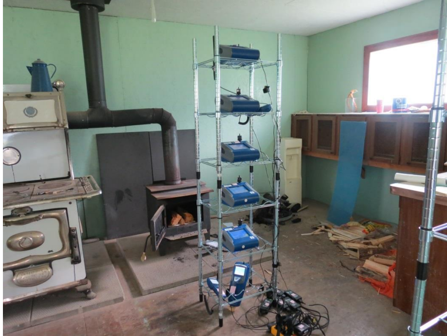
Figure 3.1. Location of Instruments used to Monitor PM 2.5 Distribution at Various Heights above Floor Level, 3' from the Woodstove
