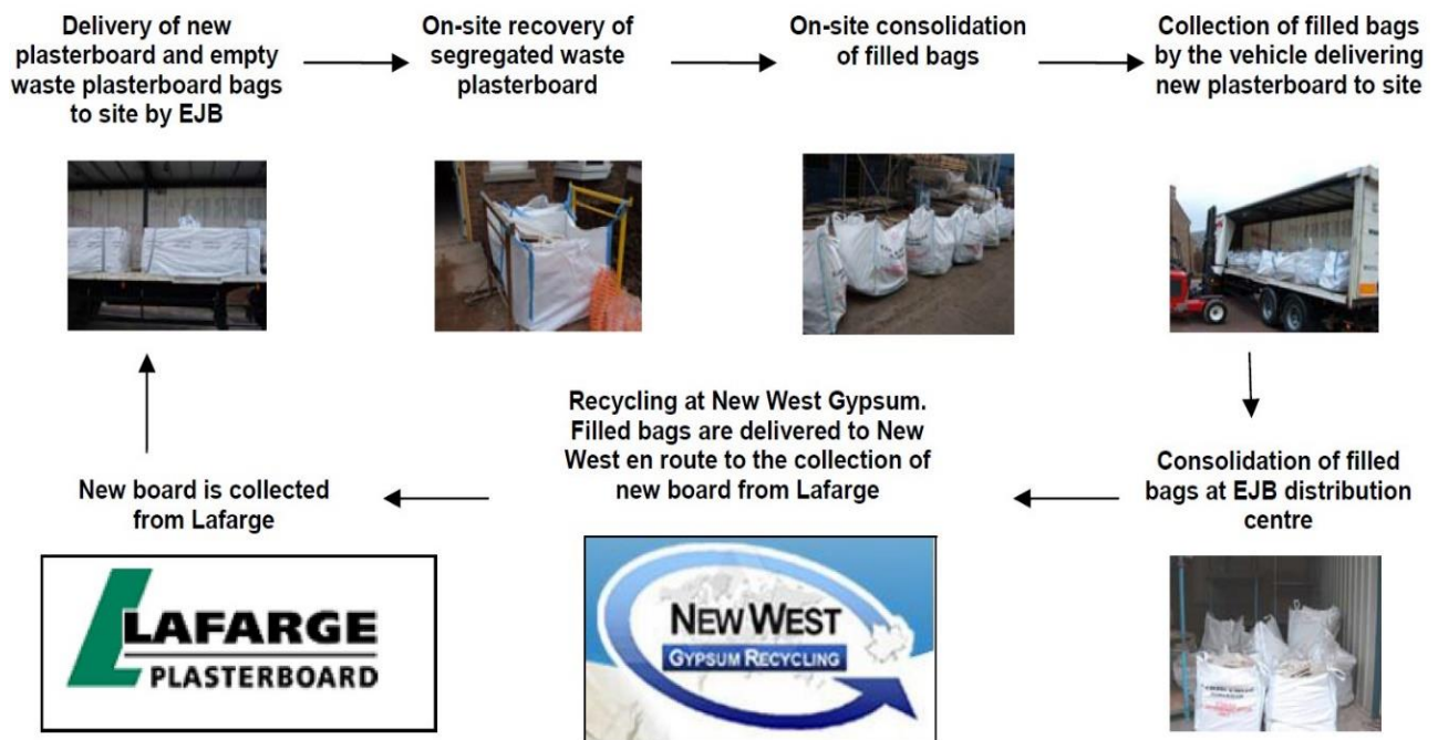
Figure 9. EJ Berry's take-back process for collecting gypsum board waste
