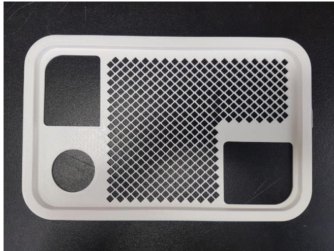
Figure 3-14- The 3D printed prototype of the designed tray for the smart cage. This prototype is printed with a different 3D printer, Fortus 400mc, at the OIC Precision Laboratories in one piece using ABS plastics.
