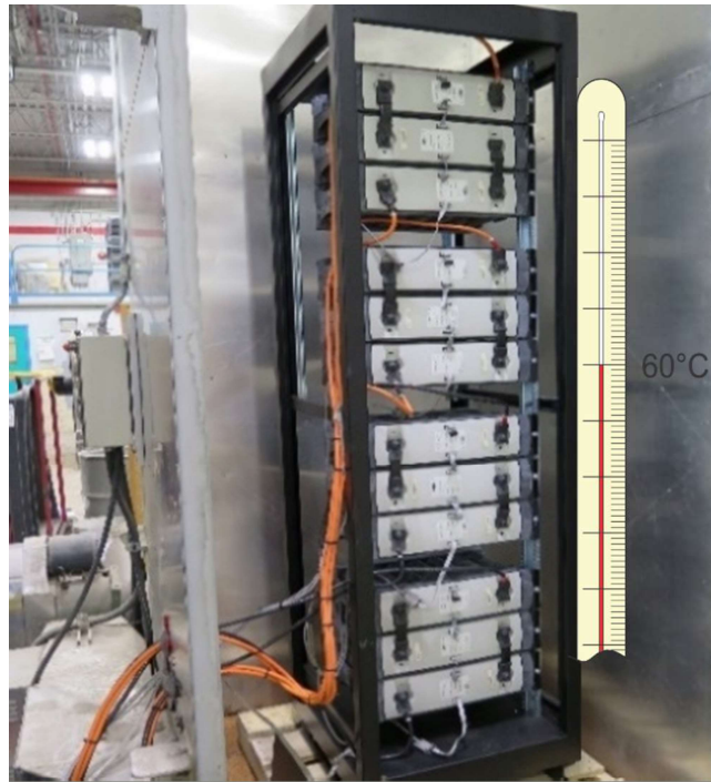
Figure 3.6 Battery strings inside oven
