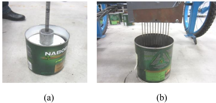
Figure 6.2. Soil preparation and cone index measurement in the laboratory: (a) container, soil and compacting proctor; (b) penetration test using the micropenetrometer.
