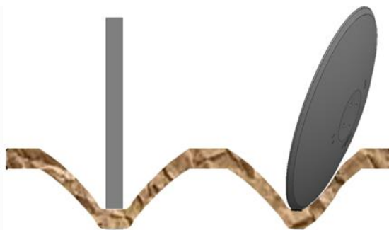
Figure 5.9. A sketch showing different soil disturbance mechanisms of a tine and disc.
