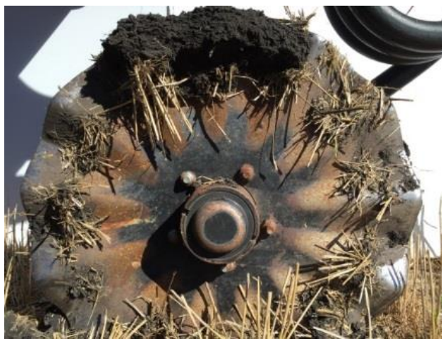
Figure 4.4. Soil and residue stuck on the coulter.
