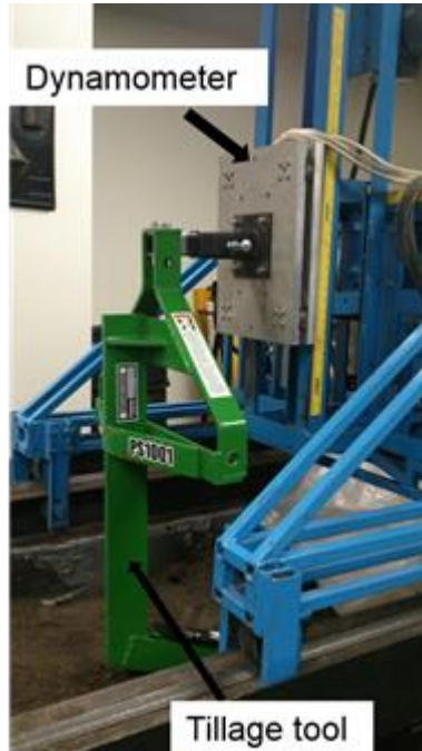
Figure 7.4. Lab test setup showing the subsoiler-type tool mounted on the tool carriage through a dynamometer.
