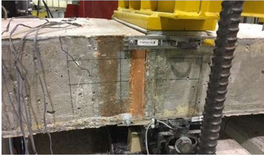
Figure 68 Image of sample number 10 after yielding of the steel reinforcement
