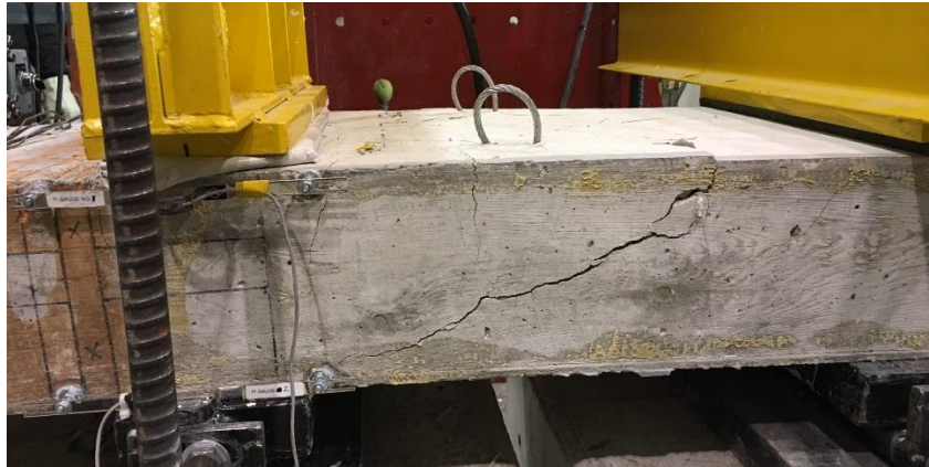
Figure 65 Concrete shear failure between support A and support B in sample 5
