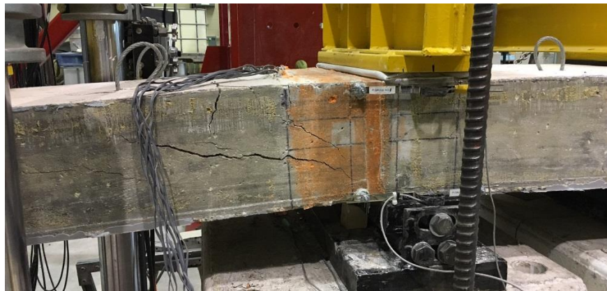
Figure 62 Concrete shear cracking immediately prior to failure in Sample 2
