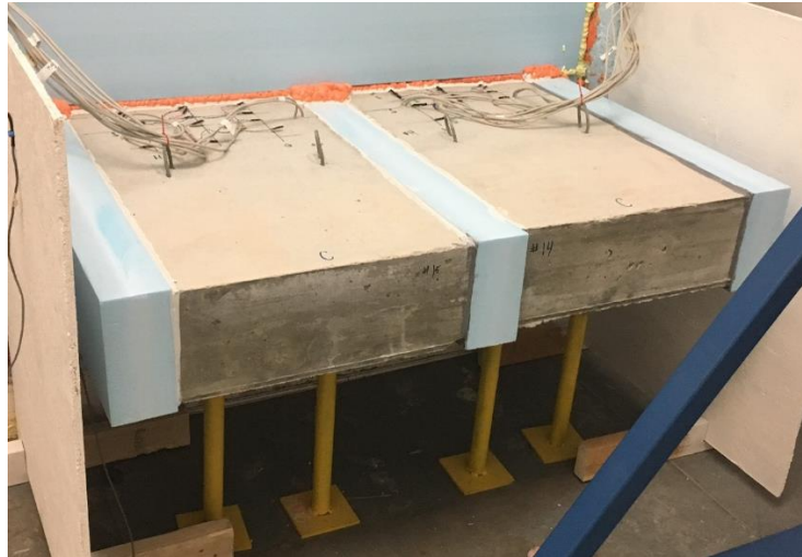
Figure 9 Test samples in thermal chamber showing longitudinal side insulation
