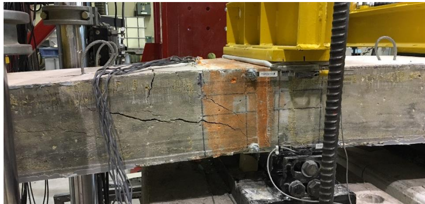
Figure 63 Concrete shear cracking to the left of Support A prior to ultimate failure in sample 3
