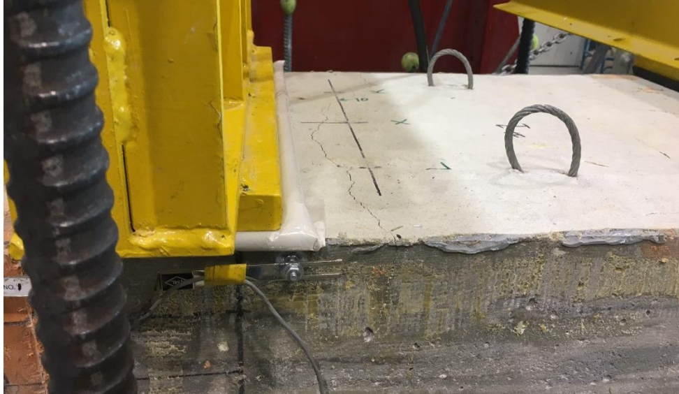
Figure 61 Concrete flexural cracking between support A and B on sample 1
