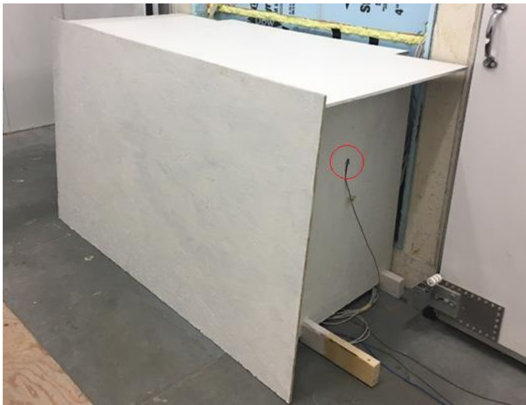
Figure 10 Plywood shelter with rear wall removed showing location of interior temperature sensor
