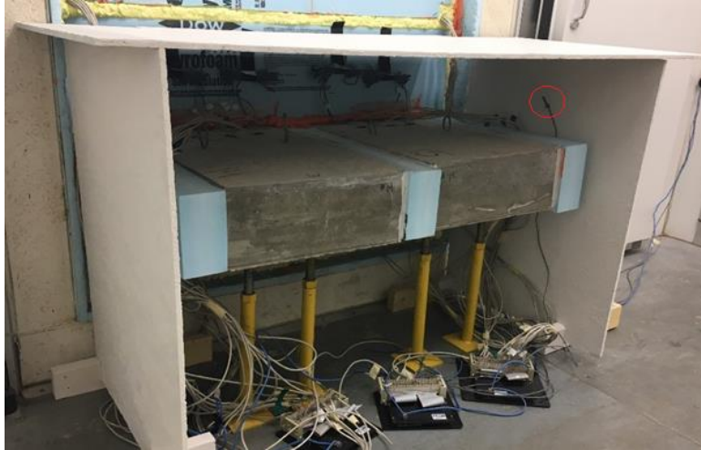
Figure 10 Plywood shelter with rear wall removed showing location of interior temperature sensor
