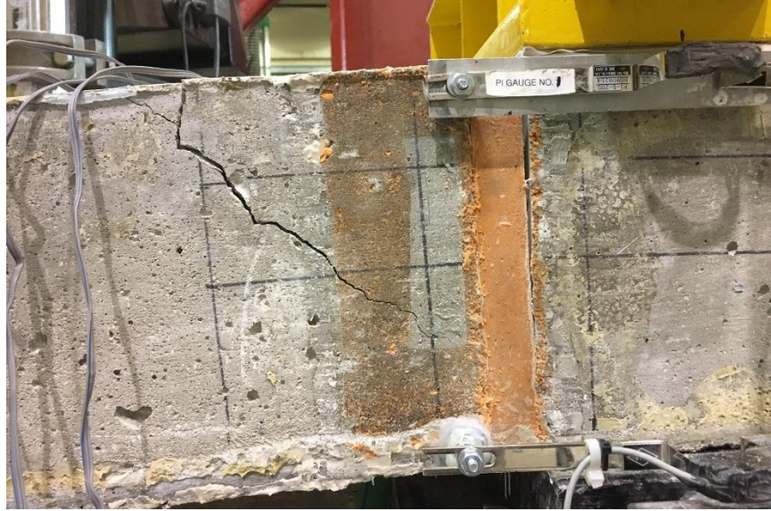
Figure 73 Sample 13 after yielding of the stainless steel reinforcement
