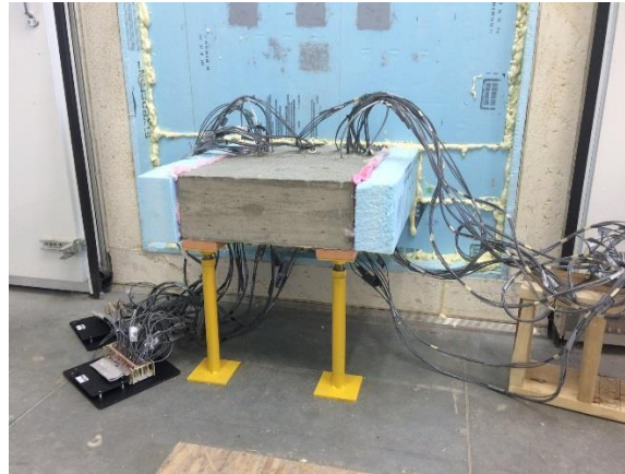
Figure 13 Mock-up thermal test on warm side
