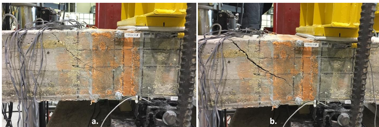
Figure 60 Concrete shear cracking in sample 1 immediately adjacent to support A between support A and the load point a) early on in testing but after ultimate design load and b) shortly before ultimate failure.
