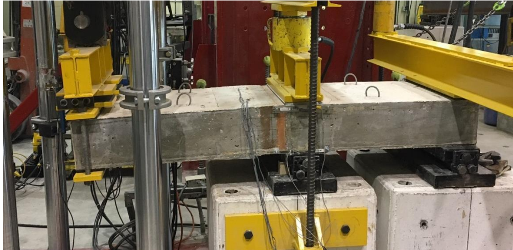
Figure 69 Deflection of sample number 10 at the end of testing
