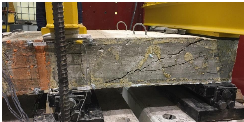
Figure 64 Concrete shear failure occurring between support A and B in sample 3
