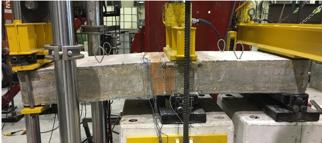
Figure 71 Figure 15 Deflection of sample number 8 at the end of testing
