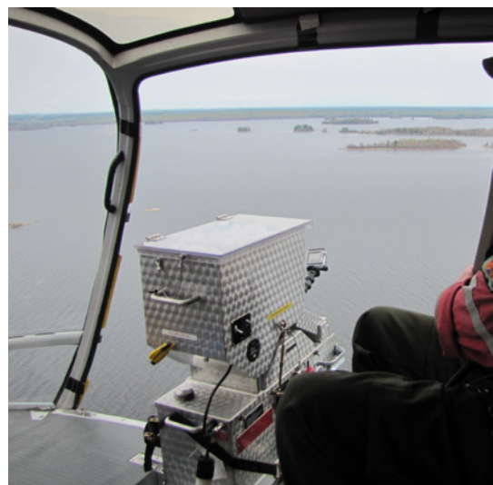
Photo 17: Premo aerial ignition device. Source: (OMNRF)
