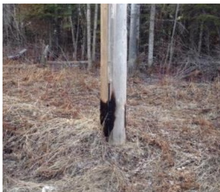
Photo 2 and 3: Fire damaged hydro pole and prescribed burn around hydro pole in WIN. Source: (OMNRF)
