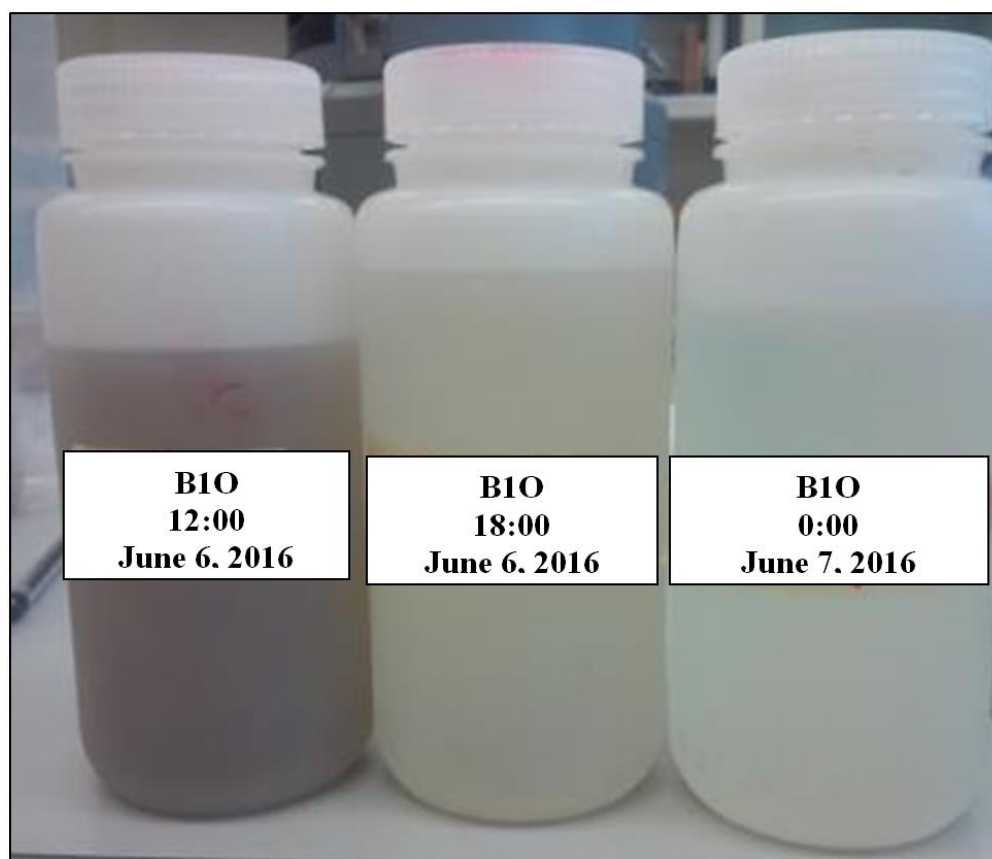
Figure 2.28. Water samples taken 6 hours apart during an event in June 2016. The turbidity of the samples decreased during the event.
