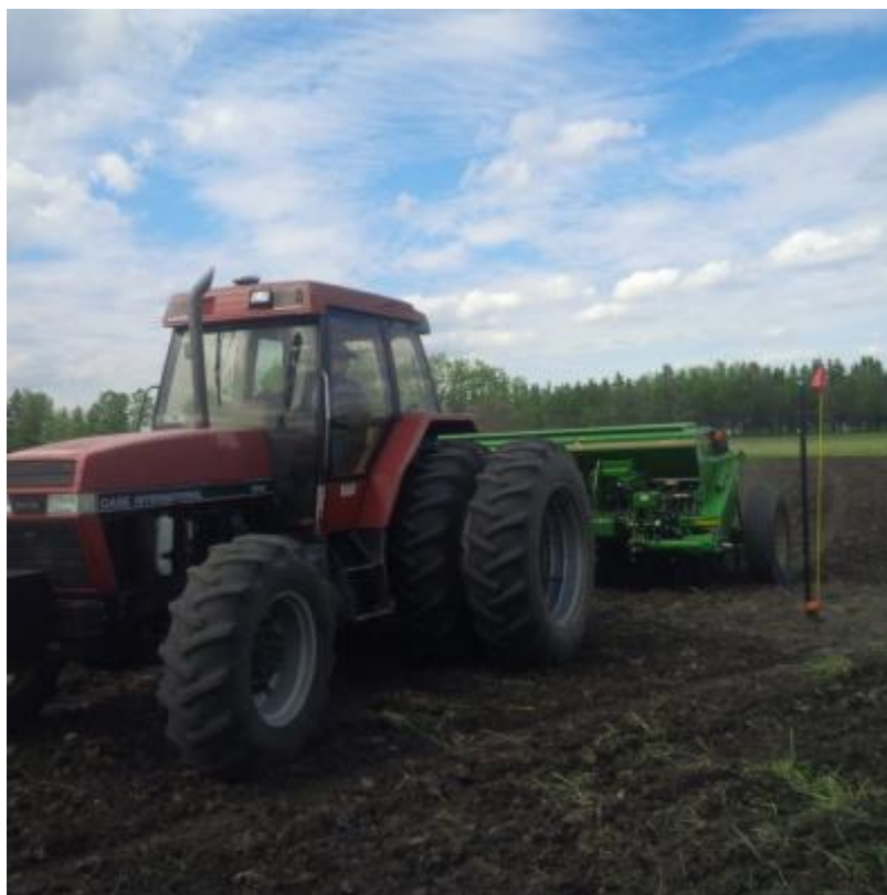
Figure 2.8. Great Plains Drill used for seeding of grasses and forbs and annual crop treatments
