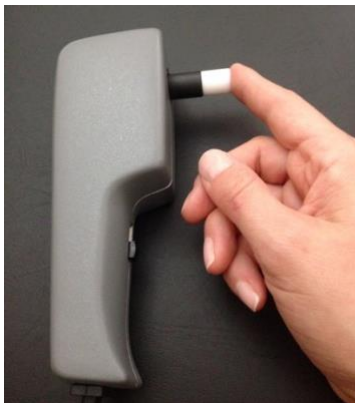
Vibration sensory analyzer for testing index finger vibration perception
