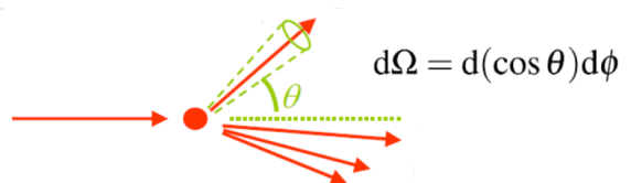
Fig. 2: Schematic description of particle beam scattering from a target, and an element of the solid angle.
