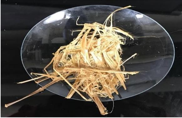
Figure 4.39 (c): *Typha* fibre from soft wood bark, 80°C/3% KOH/12 h
