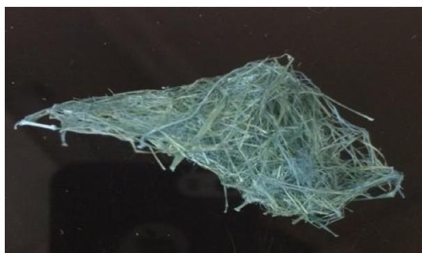
Figure 5.42: Dyed *Typha* (S8-K2-MS) fibres sample at 60°C.
