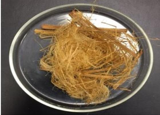
Figure 4.15 (a): Appearance of *Typha* plant treated with alkali (Sample: S8-K1-MS) for 2h at 80°C
