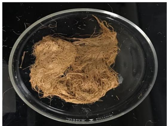
Figure 4.24 (d): *Typha* fibre treated with LiOH (Sample ID: S10-L2-NS) for 4h/3%/80°C
