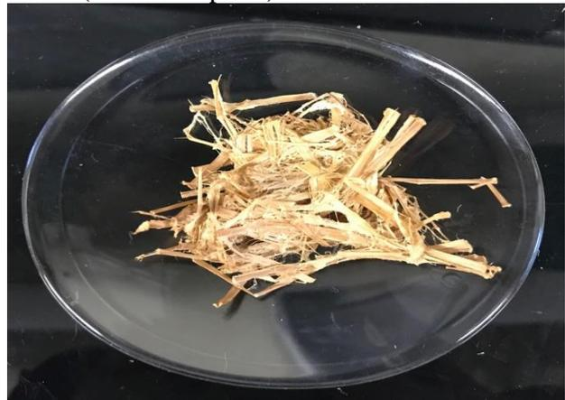
Figure 4.39 (b): *Typha* fibre from soft wood bark, 80°C/3% KOH/8 h
