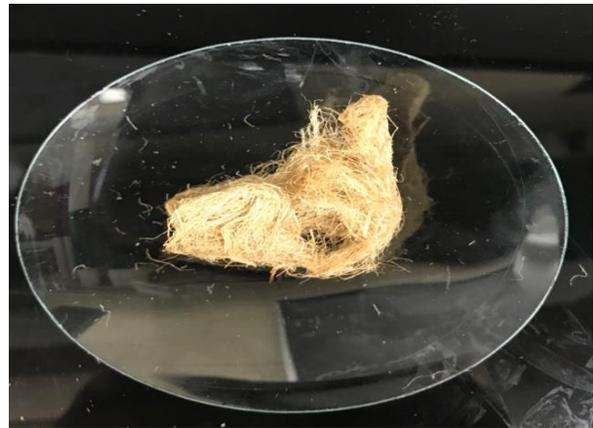
Figure 4.32 (b): Fibre from *Typha* leaves (hard stem plant)
