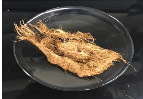
Figure 4.18 (a): Appearance of *Typha* plant treated with alkali (Sample: S8-K4-MS) for 8h at 95°C
