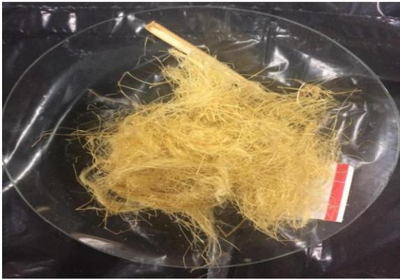
Figure 4.23 (a): Appearance of *Typha* plant treated with LiOH (Sample: S10-L1-MS) for 2h at 80°C
