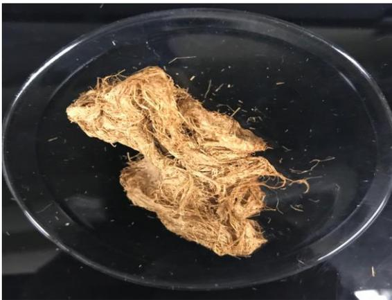
Figure 4.21 (d): *Typha* fibre treated with alkali (Sample: S9-K7-NS) for 6h/3%/95 °C
