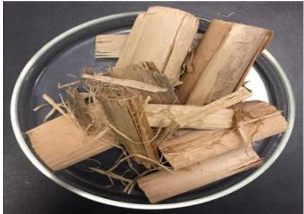
Figure 4.10: Appearance of *Typha* plant treated with alkali (Sample: S4-CH<sub>3</sub>COOH) for 2h/1%/60°C
