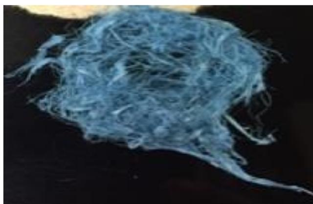
Figure 5.35: Reactive blue 4 treated *Typha* fibres. (Sample: S5-NaOH-MS/4h/80°C)
