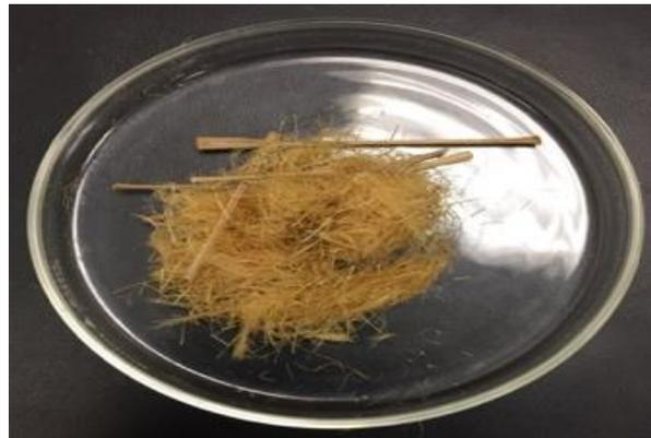
Figure 4.24 (a): Appearance of *Typha* plant treated with LiOH (Sample: S10-L2-MS) for 4h at 80°C
