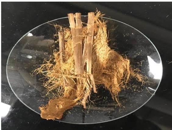
Figure 4.26 (c): *Typha* fibre treated with LiOH (Sample: S10-L4-SS) for 8h/3%/80°C
