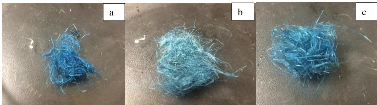
Figure 5.46: Shade variation of dyed *Typha* sample in hot plate test (a: at 60 °C) (b: less than 50 °C) and (c: 50 °C temperature).
