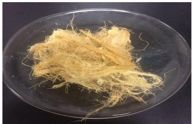
Figure 4.41 (b): Fibre from *Typha* leaves with soft spongy tissue (No stem plant), 80°C/3% KOH/8 h
