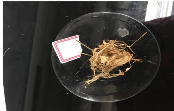
Figure 4.16 (b): *Typha* fibre treated with alkali (Sample: S8-K2-HS) for 4h/3%/80°C
