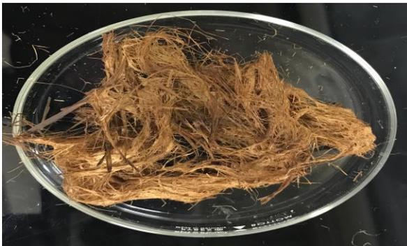
Figure 4.15 (d): *Typha* fibre treated with alkali (Sample: S8-K1-NS) for 2h/3%/80°C
