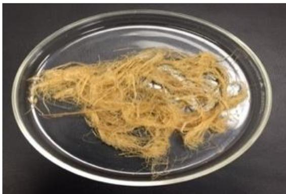
Figure 4.17 (d): *Typha* fibre treated with alkali (Sample: S8-K3-NS) for 6h/3%/80°C
