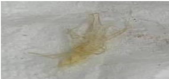
Figure 5.17(a): Virgin *Typha* fibre.
