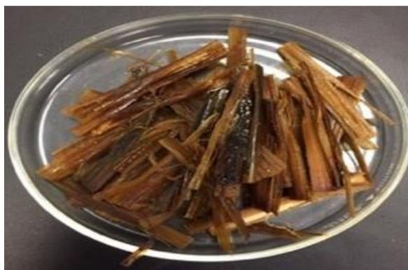
Figure 4.6: Appearance of *Typha* plant treated with alkali (Sample: S1-NaOH) for 16 days at 21°C.
