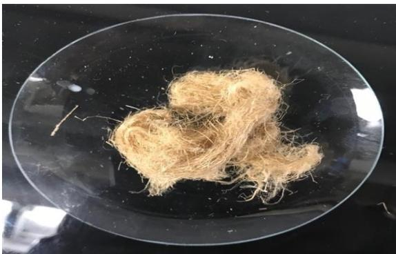
Figure 4.25 (a): Appearance of *Typha* plant treated with LiOH (Sample: S10-L3-MS) for 6h at 80°C
