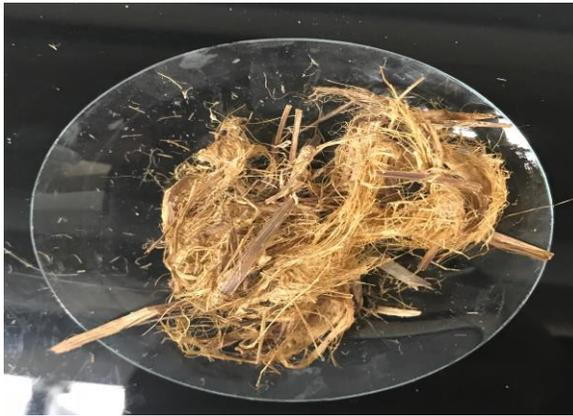
Figure 4.25 (b): *Typha* fibre treated with LiOH (Sample: S10-L3-HS) for 6h/3%/80°C
