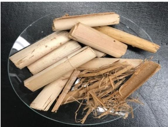
Figure 4.13: Appearance of *Typha* plant treated with acid (Sample: S7- CH<sub>3</sub>COOH) for 8h/3%/80°C
