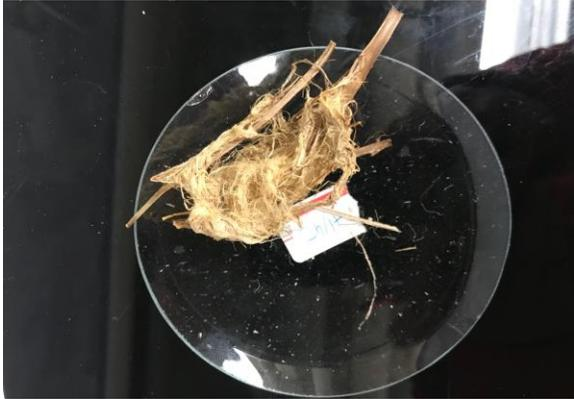
Figure 4.15 (b): *Typha* fibre treated with alkali (Sample ID: S8-K1-HS) for 2h/3%/80°C
