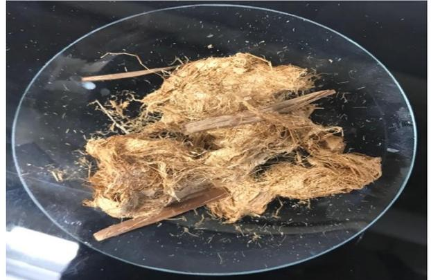
Figure 4.26 (b): *Typha latifolia* L. fibre treated with LiOH (Sample ID: S10-L4-HS) for 8h/3%/80°C
