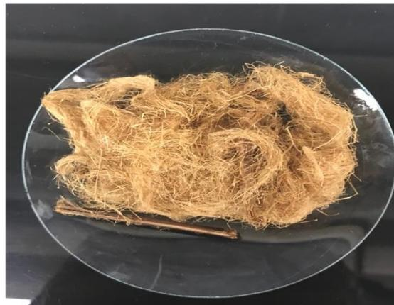
Figure 4.17 (c): *Typha* fibre treated with alkali (Sample: S8-K3-SS) for 6h/3%/80°C
