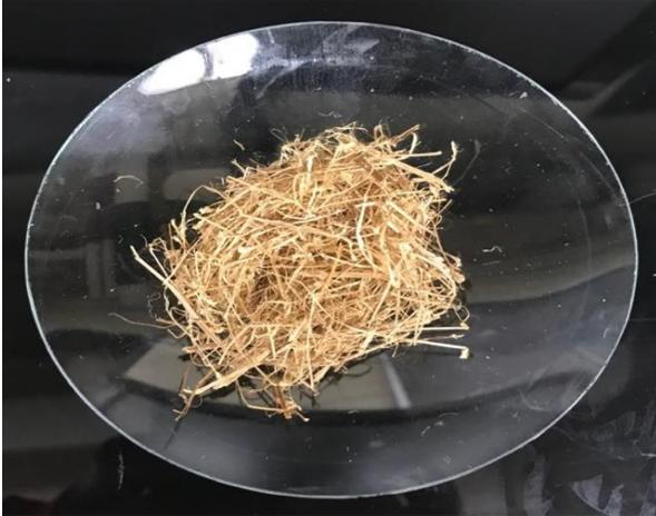
Figure 4.34 (c): *Typha* fibre from hard woody bark treated with 3% KOH for 8h
