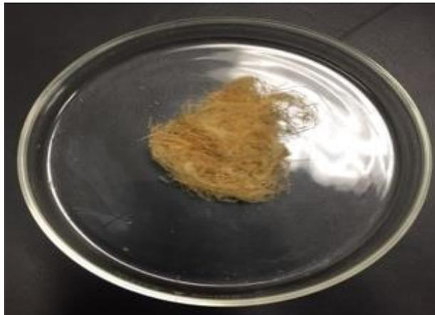
Figure 4.19 (d): *Typha* fibre treated with alkali (Sample: S9-K5-NS) for 2h/3%/95°C
