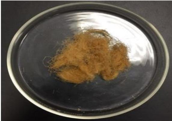
Figure 4.17 (a): Appearance of *Typha* plant treated with alkali (Sample: S8-K3-MS) for 6h at 80°C
