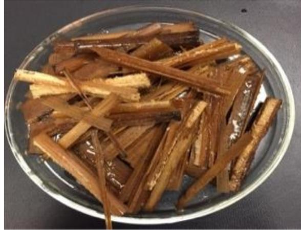
Figure 4.8: Appearance of *Typha* plant treated with enzyme (Sample: S1-Enzyme) for 16 days at 21°C
