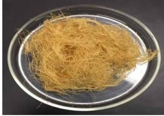
Figure 4.16 (a): Appearance of *Typha* plant treated with alkali (Sample: S8-K2-MS) for 4h at 80°C
