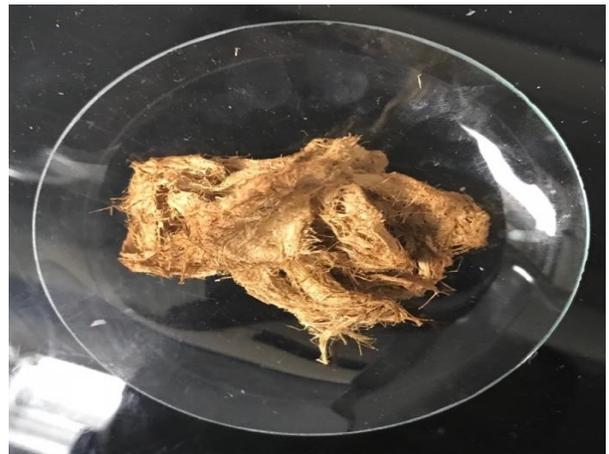
Figure 4.26 (d): *Typha latifolia* L. fibre treated with LiOH (Sample ID: S10-L4-NS) for 8h/3%/80°C
