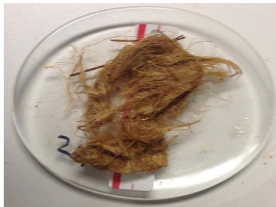
Figure 4.18 (d): *Typha* fibre treated with alkali (Sample: S9-K4-NS) for 8h/3%/80°C
