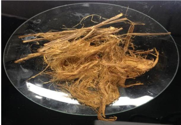
Figure 4.19 (b): *Typha* fibre treated with alkali (Sample: S9-K5-HS) for 2h/3%/95°C
