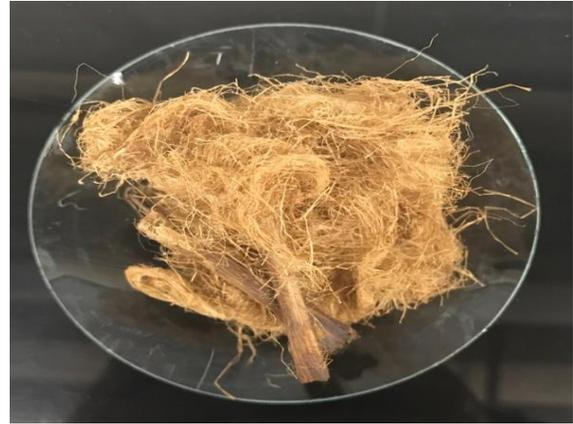
Figure 4.19 (c): *Typha* fibre treated with alkali (Sample: S9-K5-SS) for 2h/3%/95°C
