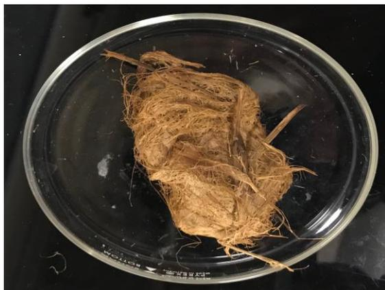
Figure 4.18 (c): *Typha* fibre treated with alkali (Sample: S9-K4-SS) for 8h/3%/80°C
