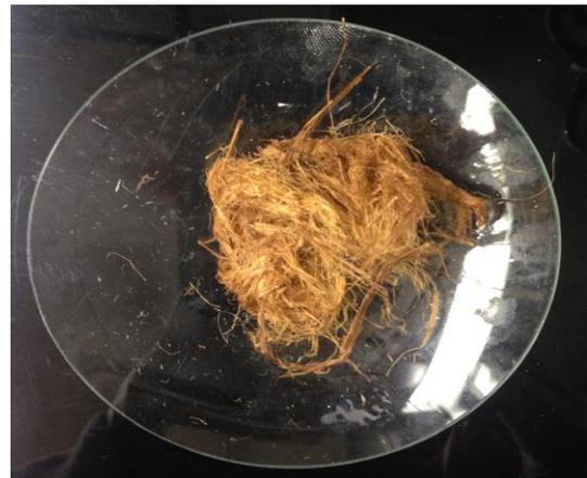
Figure 4.22 (d): *Typha* fibre treated with with KOH (Sample: S9-K8-NS) for 8h/3%/80 °C
