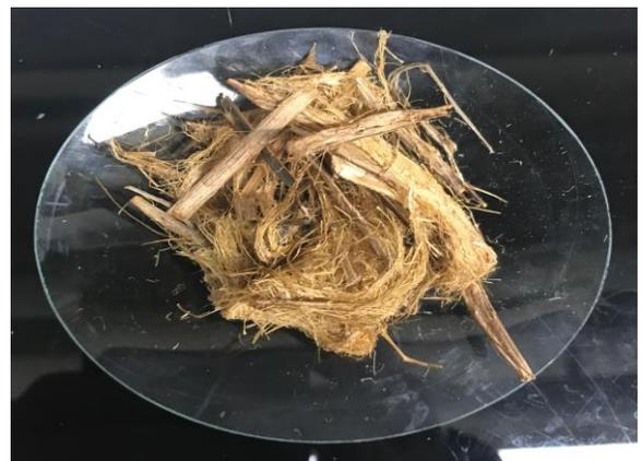
Figure 4.24 (b): *Typha* fibre treated with LiOH (Sample: S10-L2-HS) for 4h/3%/80°C
