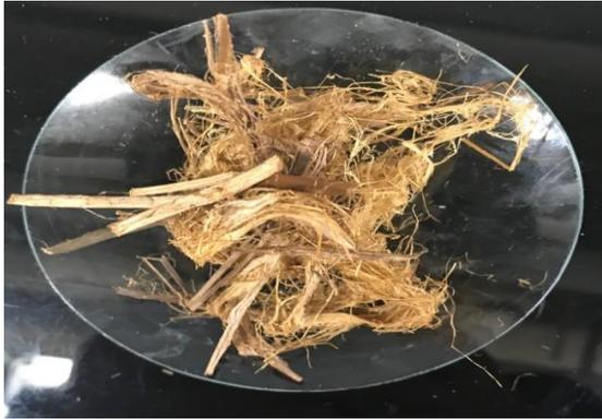
Figure 4.21 (b): *Typha* fibre treated with alkali (Sample: S9-K7-HS) for 6h/3%/95 °C
