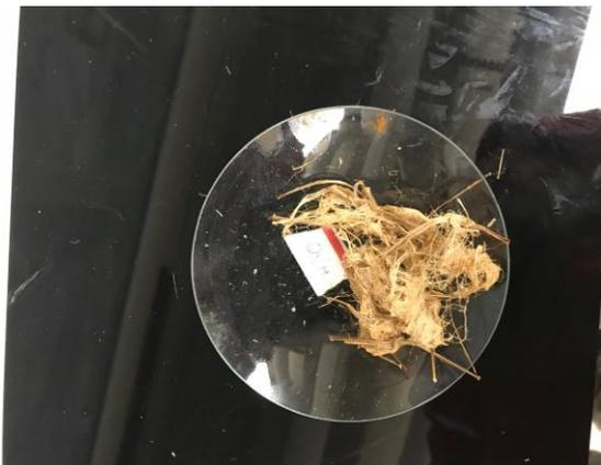
Figure 4.17 (b): *Typha* fibre treated with alkali (Sample: S8-K3-HS) for 6h/3%/80°C
