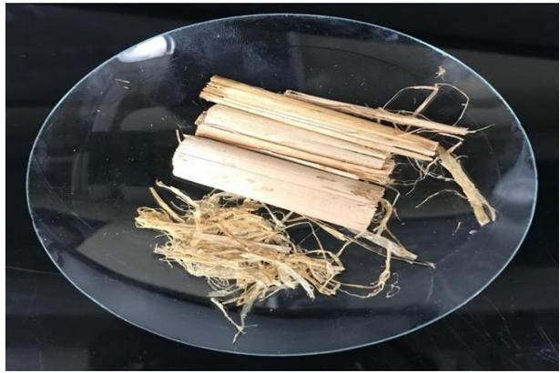
Figure 4.12: Appearance of *Typha* plant treated with acid (Sample: S6- CH<sub>3</sub>COOH) for 4h/3%/80°C
