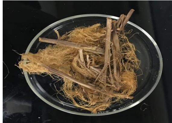
Figure 4.15 (c): *Typha* fibre treated with alkali (Sample: S8-K1-SS) for 2h/3%/80°C
