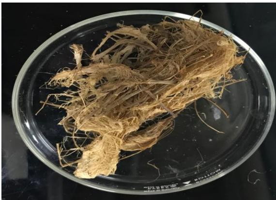
Figure 4.16 (c): *Typha* fibre treated with alkali (Sample: S8-K2-SS) for 4h/3%/80°C
