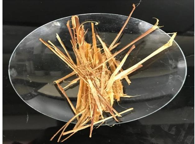
Figure 4.34 (d): *Typha* fibre from hard woody bark treated with 3% KOH for 12h.
