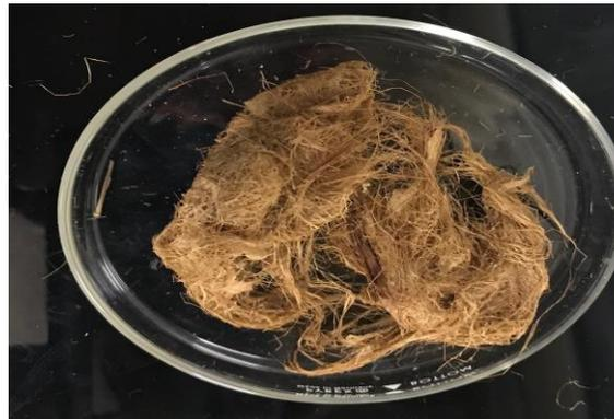
Figure 4.18 (b): *Typha* fibre treated with alkali (Sample: S8-K4-HS) for 8h/3%/80°C
