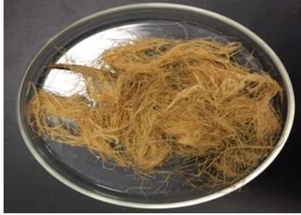
Figure 4.22 (a): Appearance of *Typha* plant treated with LiOH (Sample: S9-K8-MS) for 8h at 80°C
