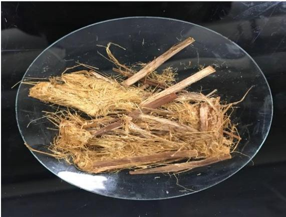
Figure 4.9: Appearance of *Typha* plant treated with alkali (Sample: S3-NaOH) for 2h/1%/60°C
