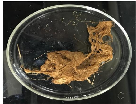
Figure 4.20 (d): *Typha* fibre treated with alkali (Sample: S9-K6-NS) for 4h/3%/95°C
