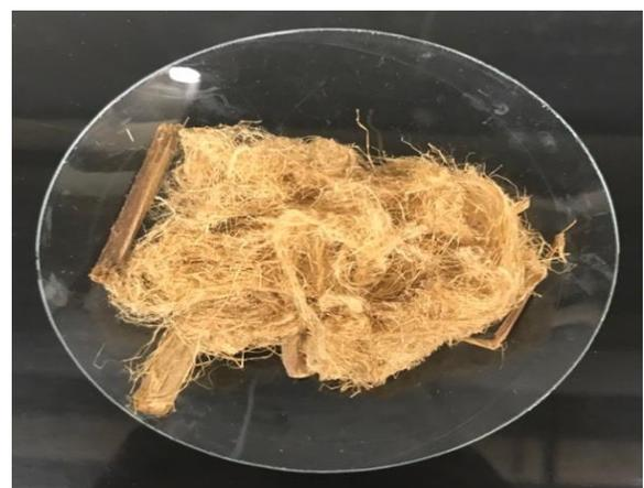
Figure 4.20 (b): *Typha* fibre treated with alkali (Sample: S9-K6-HS) for 4h/3%/95°C
