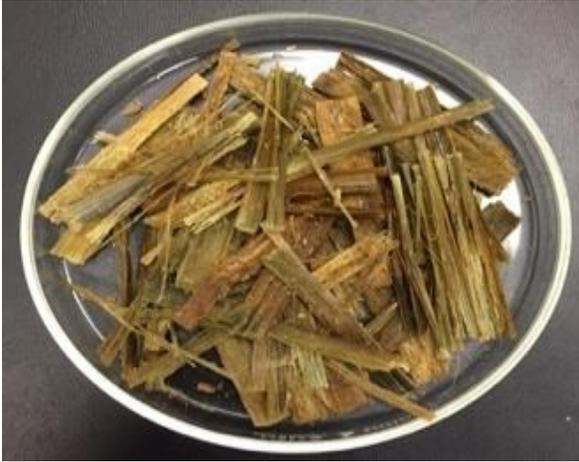
Figure 4.7: Appearance of *Typha* plant treated with alcohol (Sample: S1-CH<sub>3</sub>CH<sub>2</sub>OH) for 16 days at 21°C
