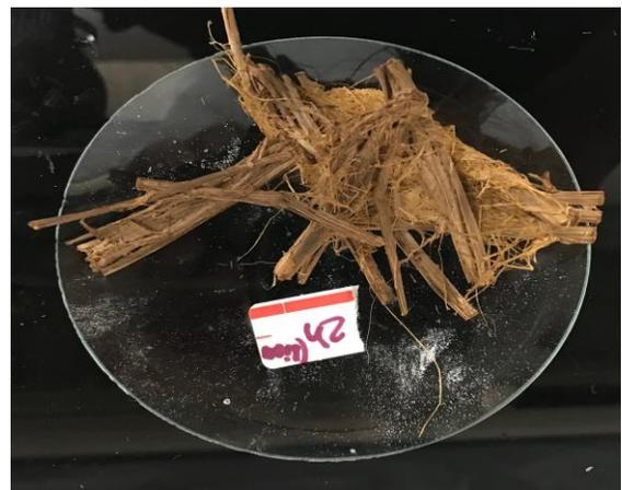
Figure 4.22 (b): *Typha* fibre treated with KOH (Sample: S9-K8-HS) for 8h/3%/80 °C
