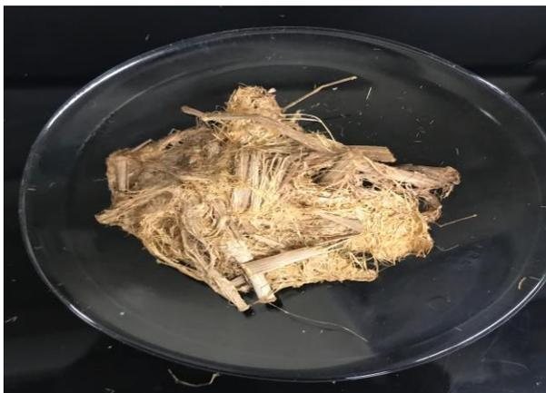
Figure 4.20 (c): *Typha* fibre treated with alkali (Sample: S9-K6-SS) for 4h/3%/95°C
