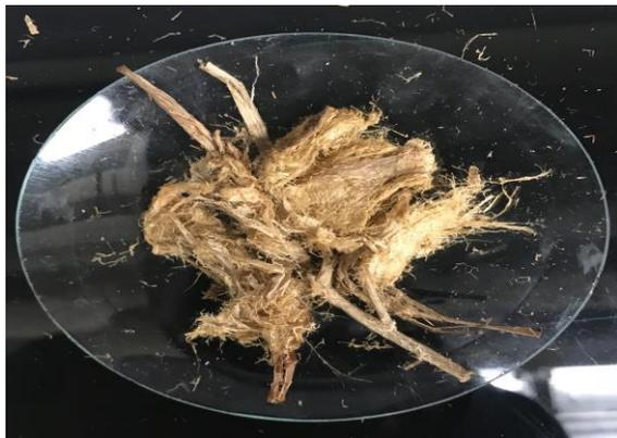
Figure 4.19 (a): Appearance of *Typha* plant treated with alkali (Sample: S9-K5-MS) for 2h at 95°C
