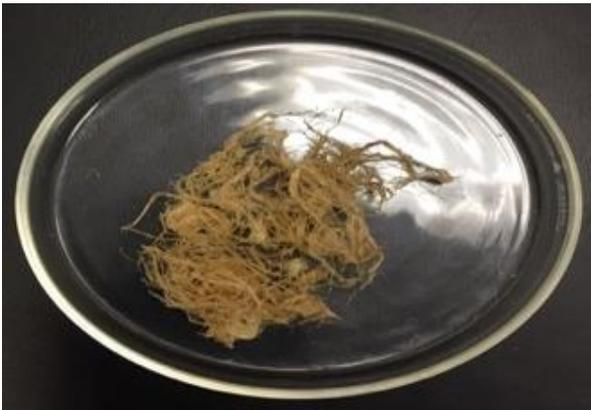
Figure 4.11: Appearance of *Typha* plant treated with alkali (Sample: S5-NaOH) for 4h/3%/80°C
