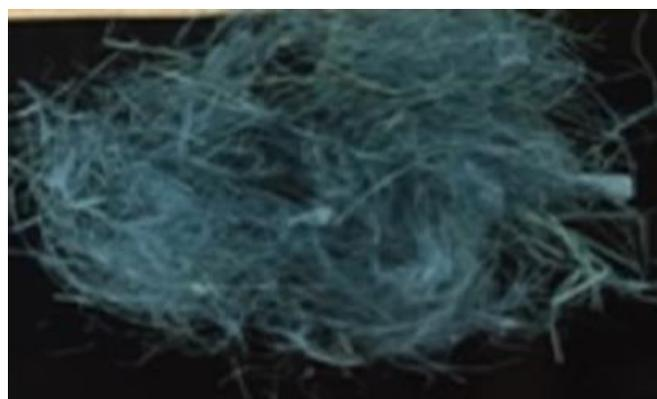
Figure 5.39: Reactive blue 4 treated *Typha* fibre (Sample: S10-L1-MS/2h/80°C).
