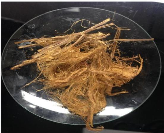
Figure 4.22 (c): *Typha* fibre treated with with KOH (Sample: S9-K8-SS) for 8h/3%/80 °C
