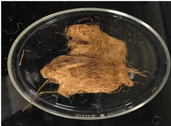
Figure 4.23 (d): *Typha* fibre treated with LiOH (Sample: S10-L2-NS) for 2h/3%/80°C
