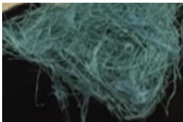
Figure 5.38: Reactive blue 4 treated *Typha* fibre (Sample: S8-K3-MS/ 6h/80°C).
