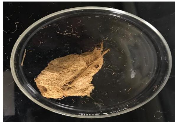
Figure 4.16 (d): *Typha* fibre treated with alkali (Sample: S8-K2-NS) for 4h/3%/80°C
