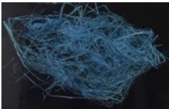
Figure 5.36: Reactive blue 4 treated *Typha* sample: S8-K2-MS/4h/80°C).
