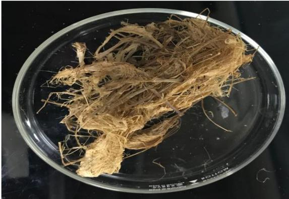
Figure 4.25 (d): *Typha* fibre treated with LiOH (Sample: S10-L3-NS) for 6h/3%/80°C
