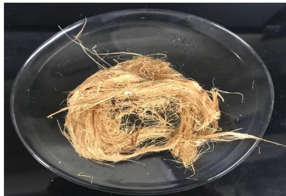
Figure 4.20 (a): Appearance of *Typha* plant treated with alkali (Sample: S9-K6-MS) for 4h at 95°C
