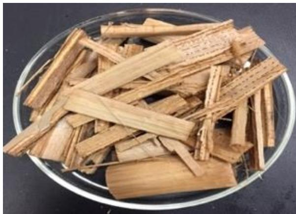
Figure 4.14: Appearance of *Typha* plant treated with Enzyme (Sample: S7-Enzyme) for 4h/3%/40°C
