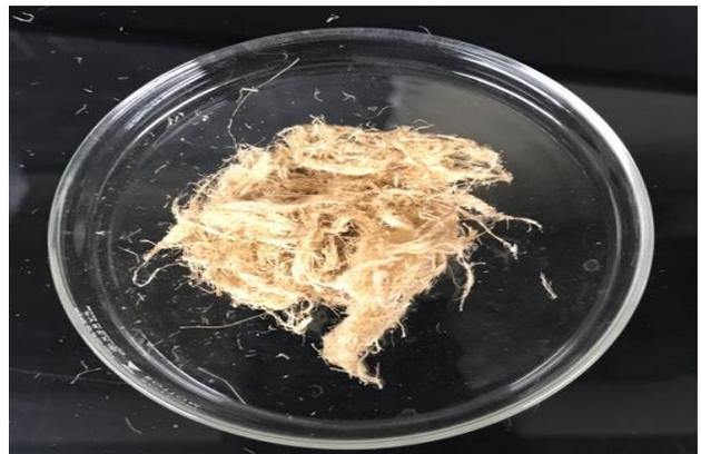
Figure 4.40 (b): Fibre from *Typha* soft spongy tissue (soft stem plant), 80°C/3% KOH/8 h
