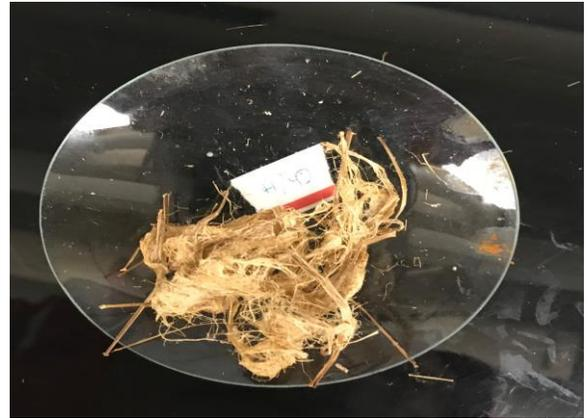
Figure 4.23 (c): *Typha* fibre treated with LiOH (Sample: S10-L1-HS) for 2h/3%/80°C
