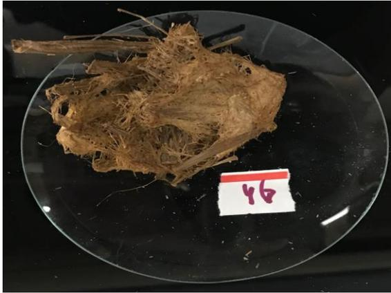
Figure 4.23 (b): *Typha* fibre treated with LiOH (Sample: S10-L1-SS) for 2h/3%/80°C
