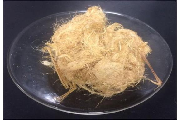
Figure 4.21 (c): *Typha* fibre treated with alkali (Sample: S9-K7-SS) for 6h/3%/95 °C
