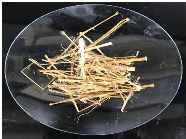
Figure 4.34 (b): *Typha* fibre from hard woody bark treated with 3% KOH for 6h.
