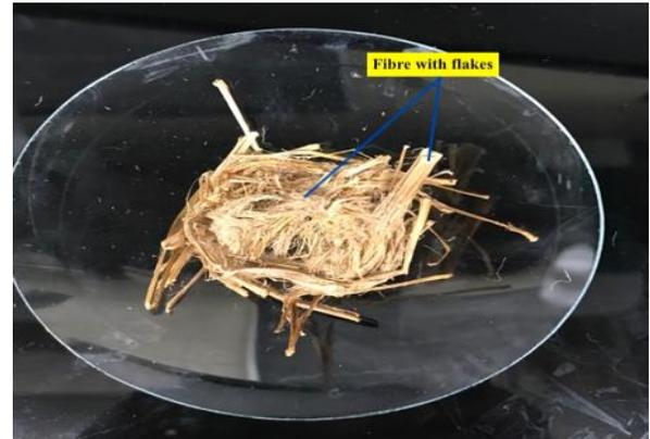
Figure 4.33 (b): Fibre from *Typha* hard wood and with spongy tissue (hard stem plant).
