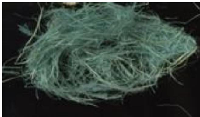
Figure 5.37: Reactive blue 4 treated *Typha* fibre (Sample: S10-L2-MS/4h/80°C).
