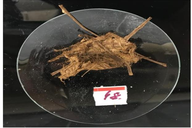
Figure 4.25 (c): *Typha latifolia* L. fibre treated with LiOH (Sample ID: S10-L3-SS) for 6h/3%/80°C
