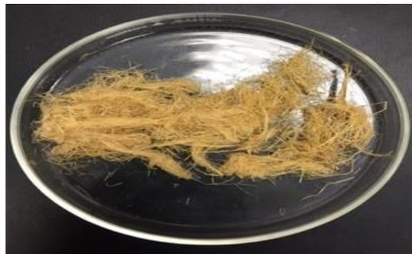
Figure 4.26 (a): Appearance of *Typha* plant treated with LiOH (Sample: S10-L4-MS) for 8h at 80°C
