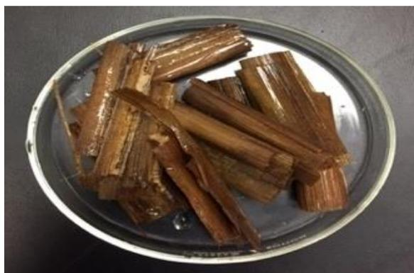
Figure 4.5: Appearance of *Typha* plant treated with acid (Sample: S1-CH<sub>3</sub>COOH) for 16 days at 21°C.
