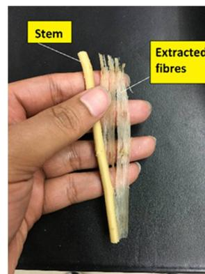
*Fig. 1.5* Canola fibre extraction from the stem.
