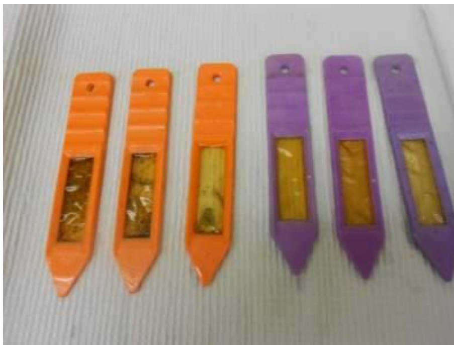
Figure 3.1 PRS TM probes retrieved from three plots from a transect, cleaned and combined to form a composite sample.
