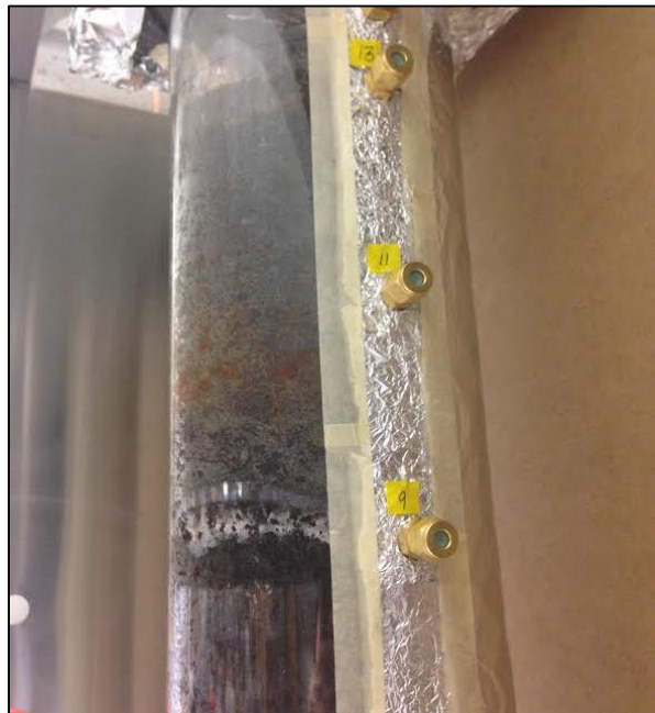
Figure 5-17: Possible EPS production in Column 2
