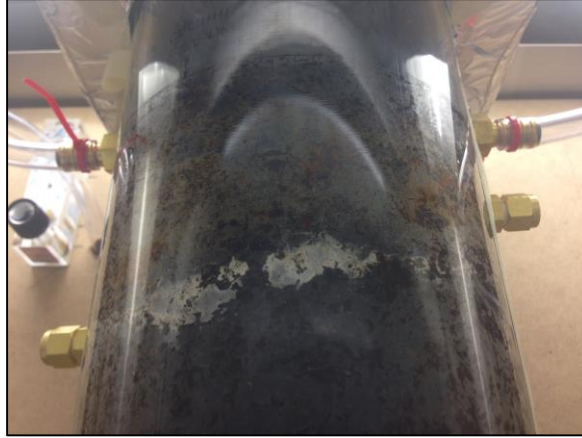
Figure 5-14: Possible EPS production in Column 1
