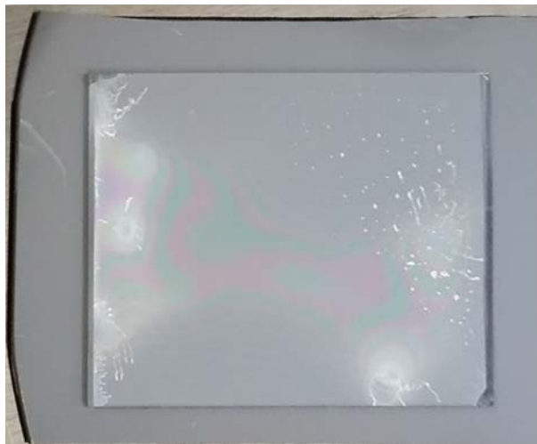
Figure 7.4: Photo of bonded Sn coated silicon wafer and 2.5 cm × 3.7 cm slide glass.
