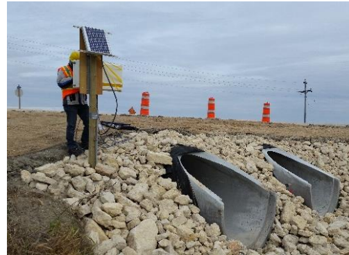
Figure 3.6: On site data download from the Campbell scientific data-logger
